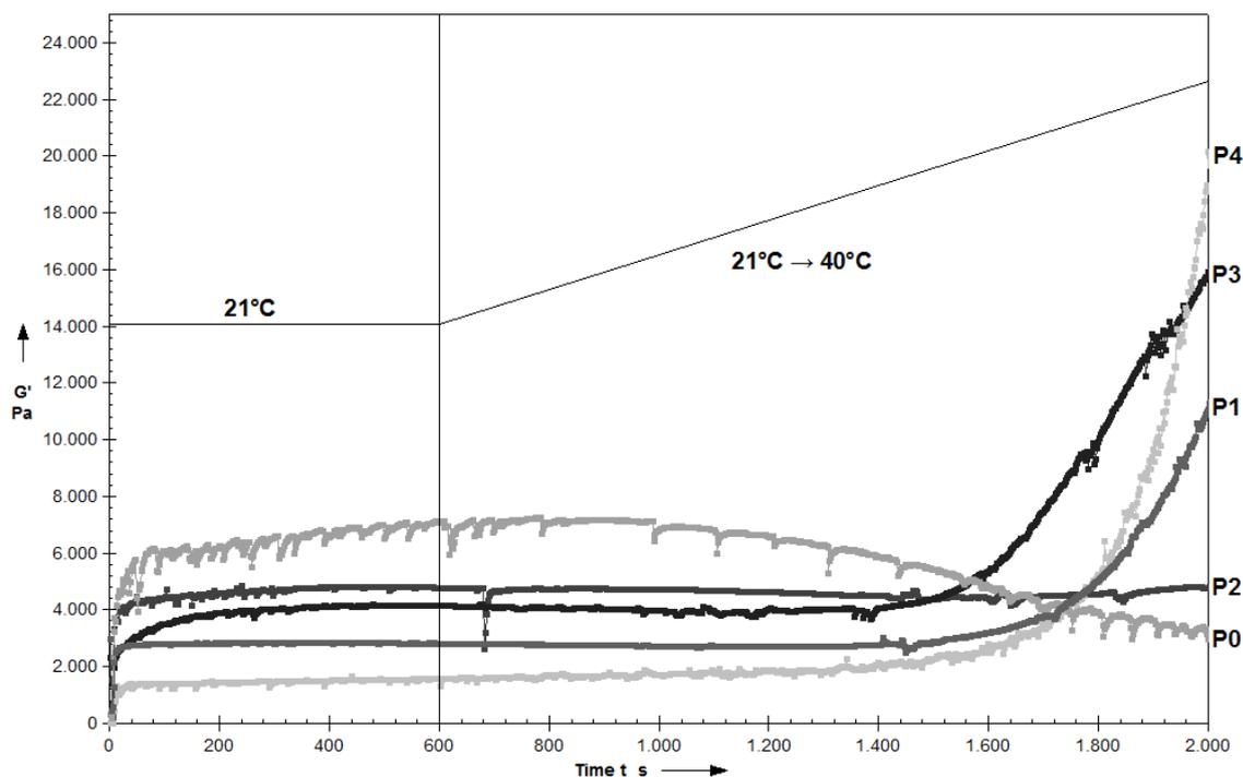
Fig. 3. Mechanical properties of hydrogel films (as recorded using a NF of 1 N). The films were UV irradiated for 60 minutes prior to investigation.
