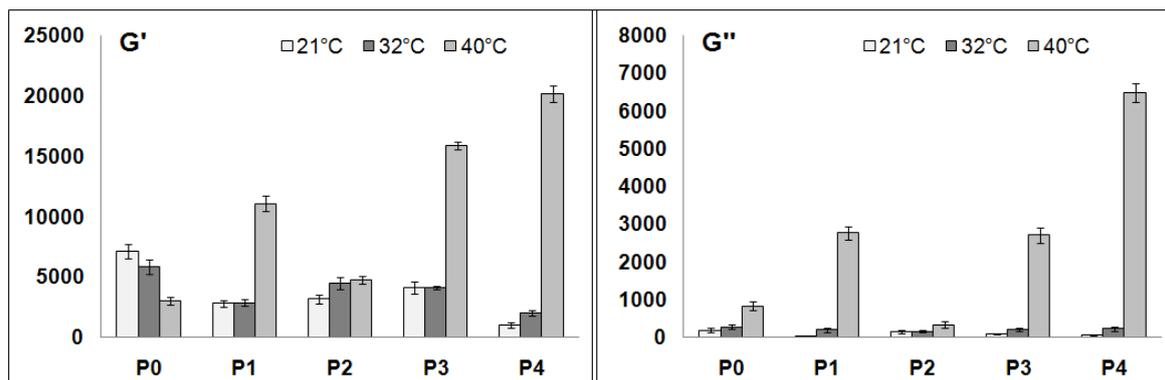
Fig. 4. Storage moduli (left) and loss moduli (right) recorded at 21, 32 and 40 °C for all obtained materials.
