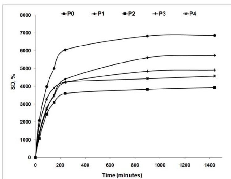
Fig. 2. Water uptake capacity expressed as SD (%) as a function of the incubation time, for the hydrogels P1–P4, when compared to the control sample, P0.
