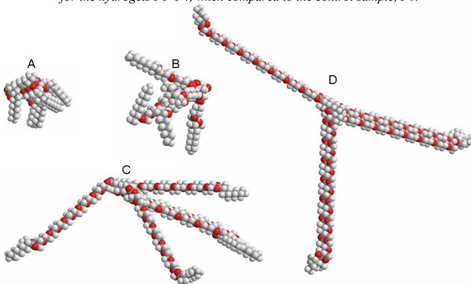
Scheme 3. Crosslinker-rich domains in the hydrogel matrices (five molecules associated through C-C chains): A – EGDMA; B – TEGDMA; C – PEGDMA I; D – PEGDMA II.
