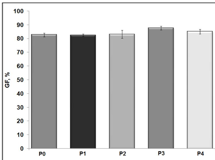
Fig. 1. GF average values for the new types of hydrogels: P0 – MAG; P1 – MAG-EGDMA; P2 – MAG-TEGDMA; P3 – MAG-PEGDMA I; P4 – MAG-PEGDMA II.
