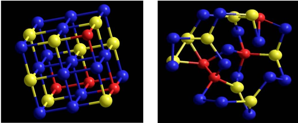
Fig. 1. The commuton a) Crystalline state (ON state) b) Amorphous state (OFF state)
