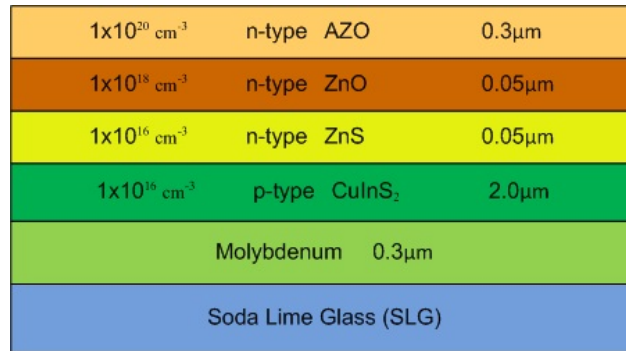
Fig. 1. Schematic diagram of CuInS 2 photovoltaic layer structure
