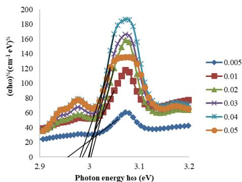
Fig. 8. Plot of  $(\alpha h\nu)^{1/2}$  against photon energy  $h\nu$  of samarium NPs doped tellurite glass.
