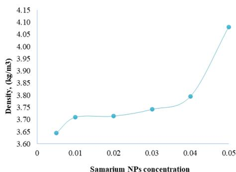
Fig. 4. Density of samarium NPs doped tellurite glass.
