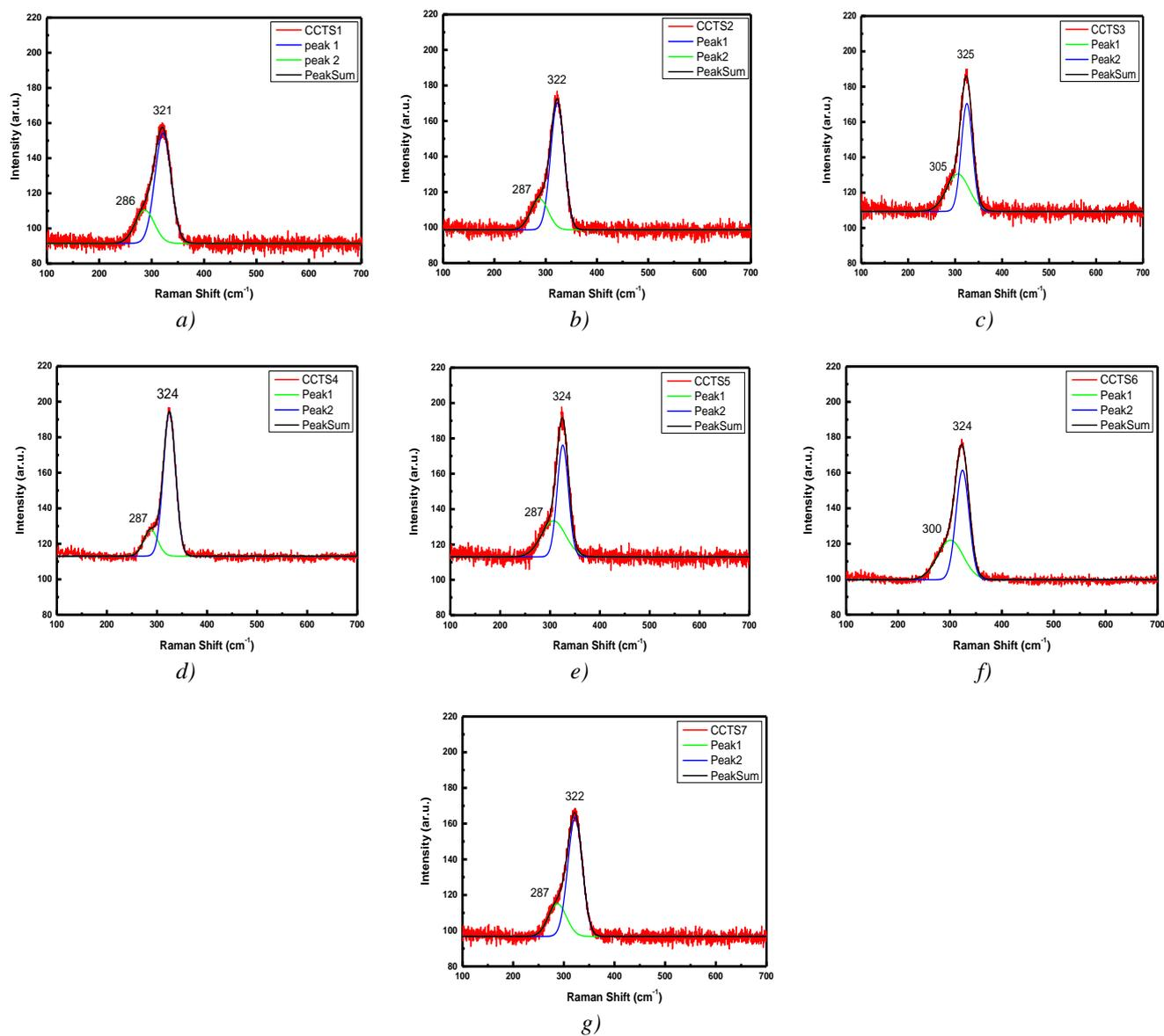
Fig. 3 Raman spectrum for thin film of a) CCTS1; b) CCTS2; c) CCTS3; d) CCTS4; e) CCTS5; f) CCTS6; and g) CCTS7
