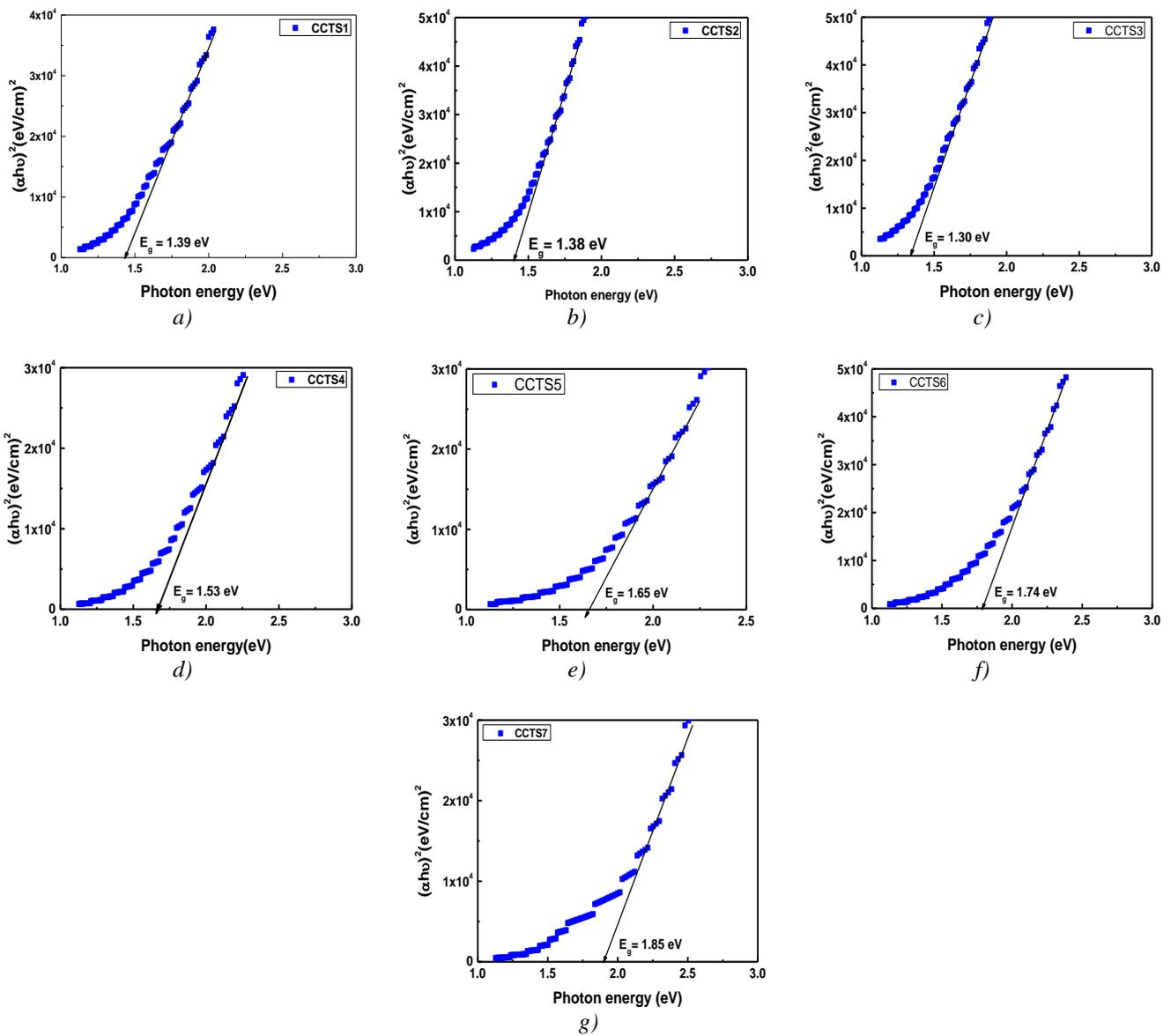
Fig. 5 g. The relation between  $(ah\nu)^2$  and  $(h\nu)$  for thin film of a) CCTS1; b) CCTS2; c) CCTS3; d) CCTS4; e) CCTS5; f) CCTS6; and g) CCTS7
