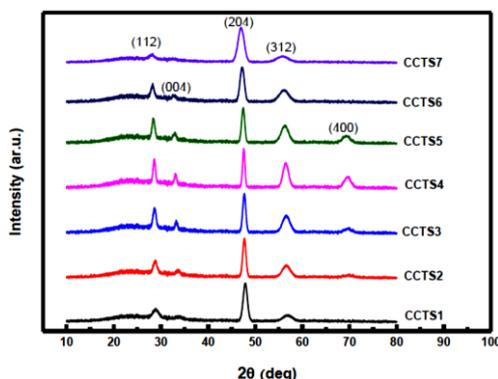
Fig. 2. X-ray diffraction patterns of CCTS thin films
