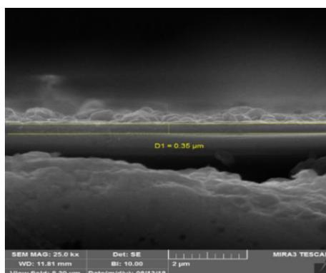
Fig. 1. Cross section image of typical CCTS film.
