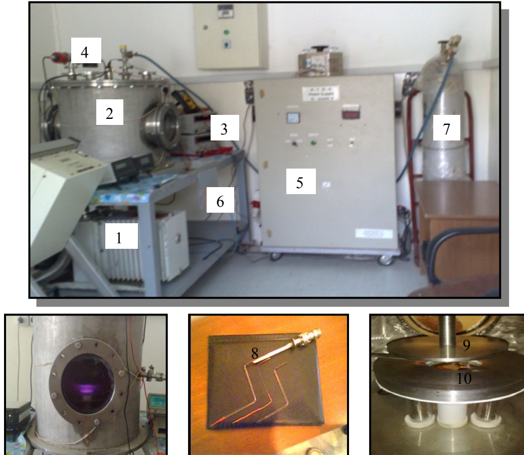
Fig. 2. Low pressure (dc-glow discharge) plasma system.
