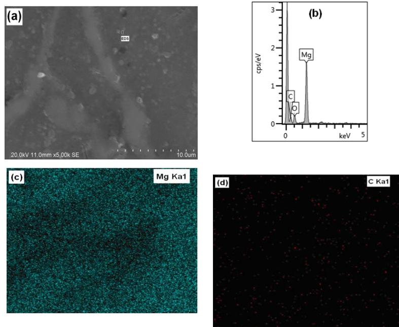
*Fig. 7 (a) SEM image of composite surface with 1.5 wt.% graphene nano-sheets; (b) the EDS of the selected area in (a); (c-d) SEM mapping of composite: (c) magnesium; (d) graphene nano-sheets.*
