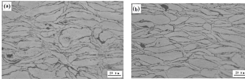
*Fig. 5 The microstructures of the composites with different graphene content and ball-milling time (a) 1.5 wt.% for 72h, (b) 2.5 wt.% for 96h.*
