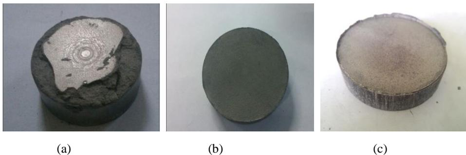
Fig.2 the sintered composite with 0.5 wt.% graphene content for different sintering temperature: (a) 560 $^{\circ}\text{C}$ , (b) 595  $^{\circ}\text{C}$  and (c) 610  $^{\circ}\text{C}$ .
