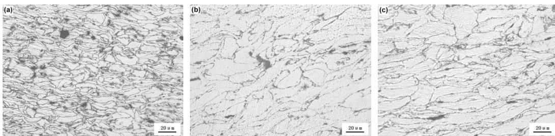
*Fig.8 The microstructures of as-rolled composite with 1.5 wt.% graphene content under different aging time, (a) 1h, (b) 2h and (c) 3h.*
