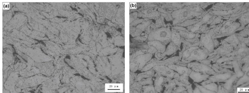
*Fig. 4 The microstructures of the composites with different graphene content for ball-milling time of 6h, (a) 1.5 wt.%, (b) 2.5 wt.%.*
