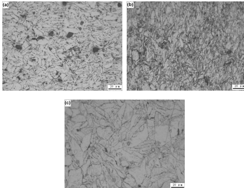
*Fig.3 The microstructures of the composites with different graphene content ball-milling time for graphene content of 0.5%, (a) 2h, (b) 4h, and (c) 6h.*
