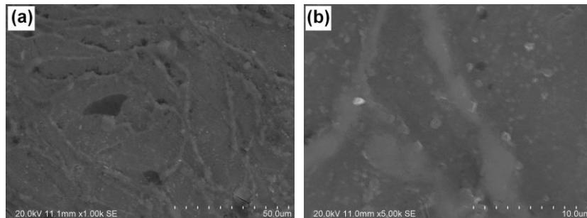
*Fig.6 The SEM images of composite with 1.5 wt.% graphene nano-sheets, (a) low-time, (b) high-time.*
