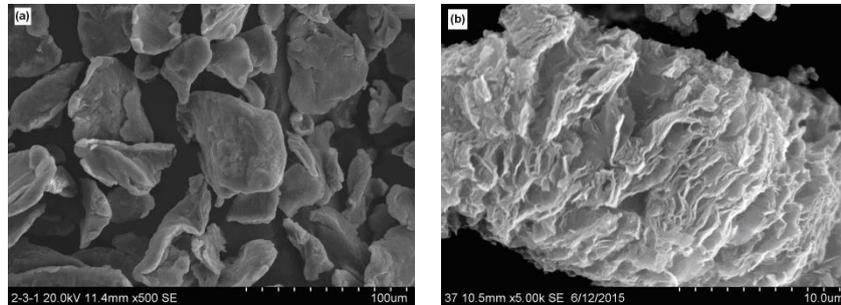
Fig. 1. SEM micrograph of powders used, (a) pure magnesium powder, (b) Graphene nano-sheets
