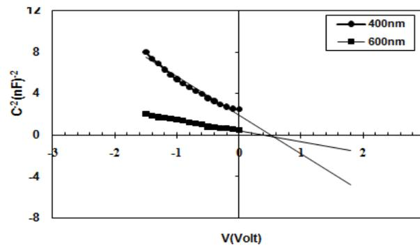
Fig.5 The variation of  $1/C^2$  as a function of reverse bias voltage PbS/Si HJ at different thickness.
