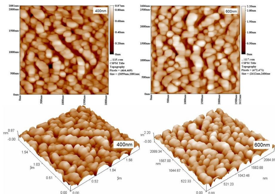
Fig. 2. Two and three-D of AFM of PbS thin films with different thicknesses (400, 600)nm.
