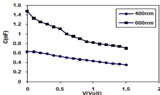
Fig.4. The variation of capacitance as a function of reverse bias voltage for PbS/Si HJ at different thickness
