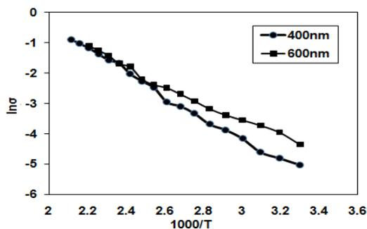
Fig. 3 The  $\ln \sigma$  versus  $1000/T$  for for PbS thin films at different thickness.
