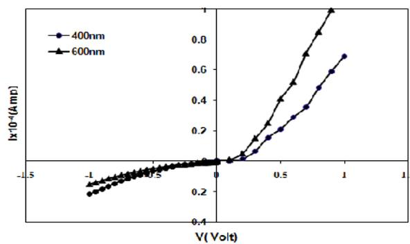
Fig. 6. The I-V characteristics for PbS/Si HJ at forward and reverse bias voltage at different thickness.
