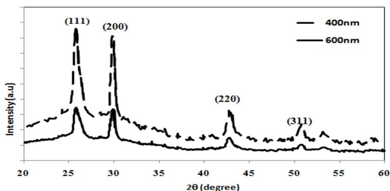
Fig. 1. The X-ray diffraction for PbS thin films at different thickness.
