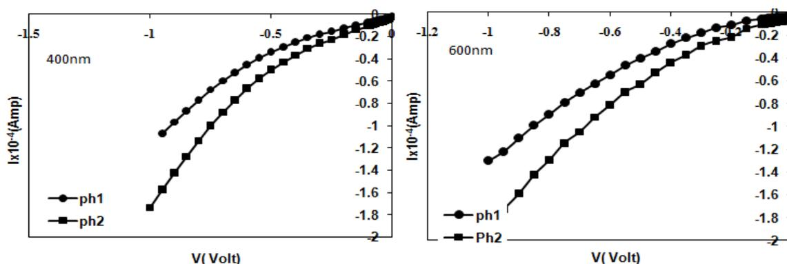
Fig. 7. *I-V characteristics under illumination for PbS/Si HJ at different thickness*
