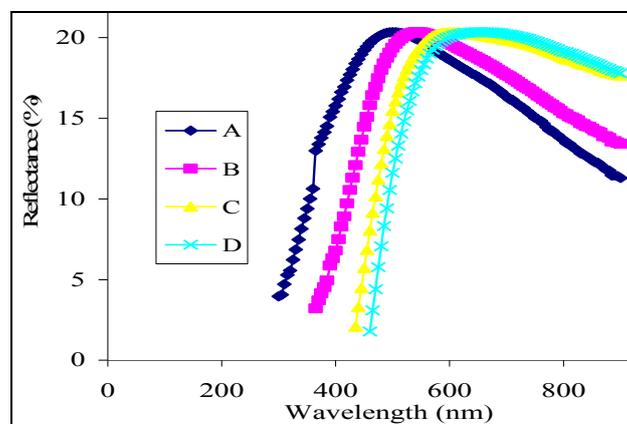
Fig.6. Reflectance vs. wavelength for PbSe thin films annealed at different temperature.
