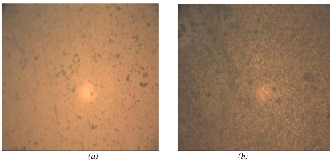
Fig.2: Photomicrograph of PbSe thin films annealed at (a)  $100^\circ\text{C}$  and (b)  $300^\circ\text{C}$
