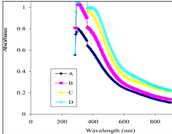
Fig.4. Absorbance vs. wavelength for PbSe thin films annealed at different temperatures.
