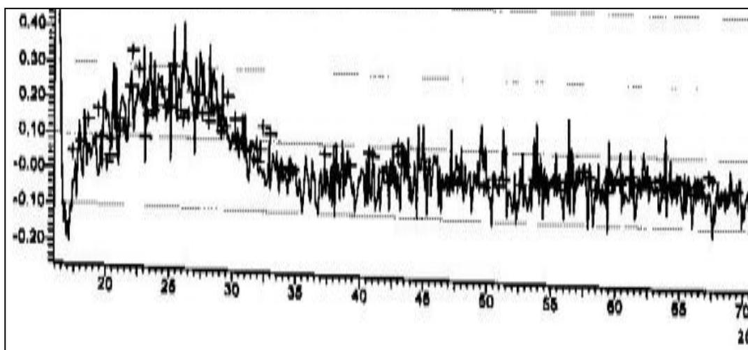
Fig. 1. XRD pattern of PbSe thin film annealed at 200 °C
