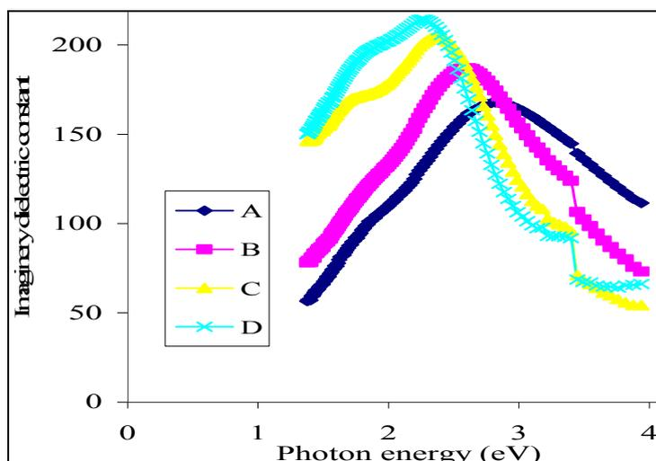
Fig.12. Imaginary dielectric constant vs. photon energy for PbSe thin films annealed at different temperatures.
