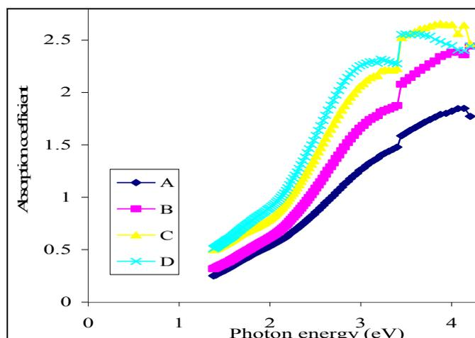
Fig.7. Absorption coefficient vs. photon energy for PbSe thin films annealed at different temperatures.
