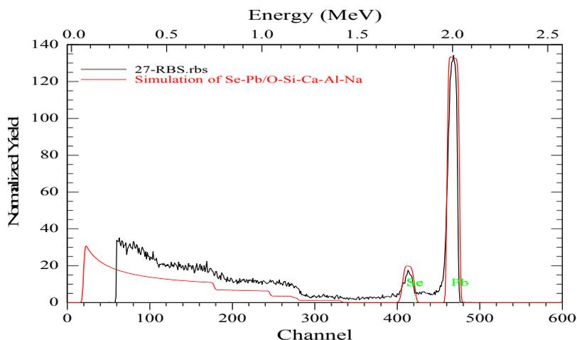
Fig. 3. RBS result for PbSe thin film annealed at  $200^\circ\text{C}$ .
