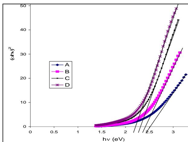
Fig. 8. Direct band gap plot for PbSe thin films annealed at different temperature.
