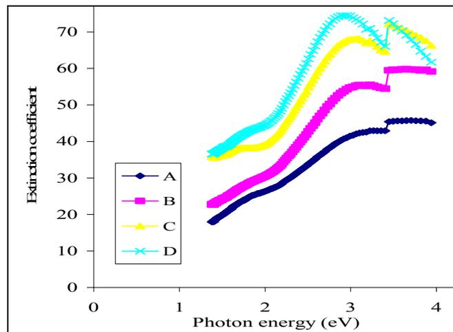
Fig.10. Extinction coefficient vs. photon energy for PbSe thin films annealed at different temperatures
