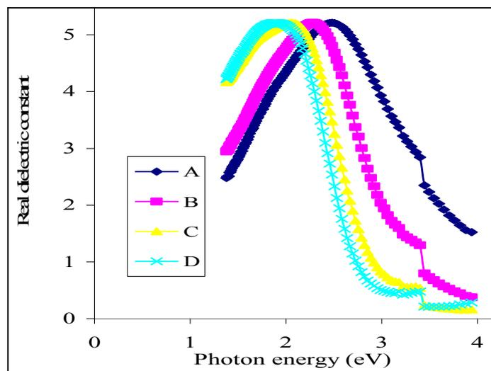
Fig.11. Real dielectric constant vs. photon energy for PbSe thin films annealed at different temperatures.
