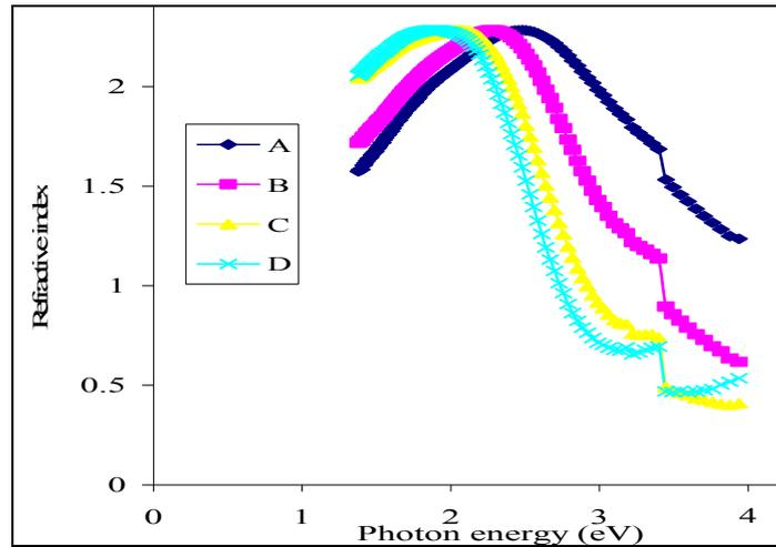
Fig. 9. Refractive index vs. photon energy for PbSe thin films annealed at different temperatures.
