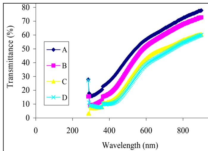
Fig. 5. Transmittance vs. wavelength for PbSe thin films annealed at different temperature.
