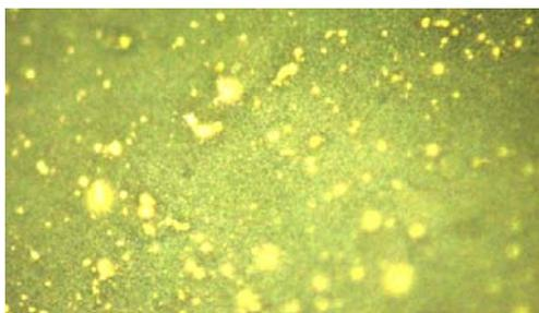
Fig. 1. Morphology of as-grown film (1000X)
