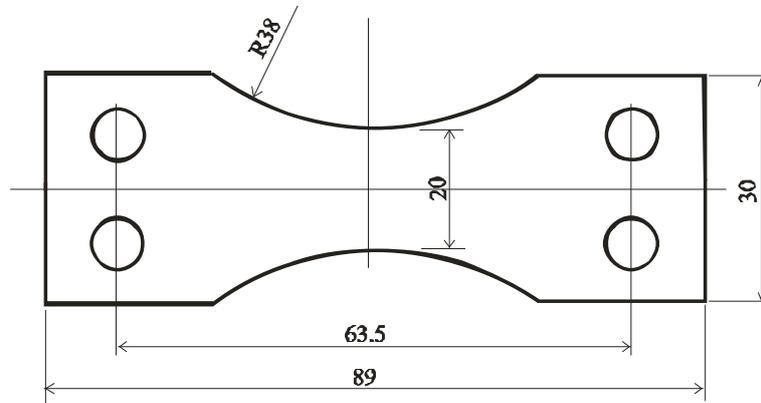
Fig. 1 The schematic drawing of the fatigue test specimen.
