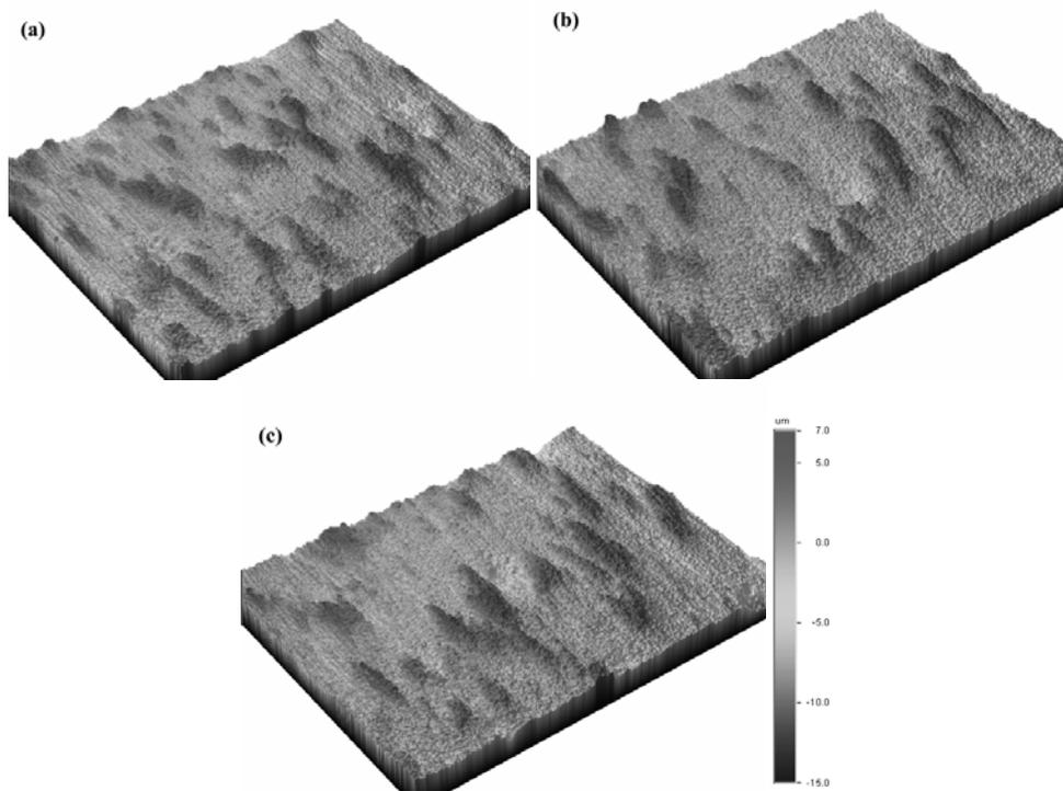
Fig. 4. Surface topographies of the as-received samples a) chemically non-treated, b) alkaline treated, c) hydrogen peroxide treated.
