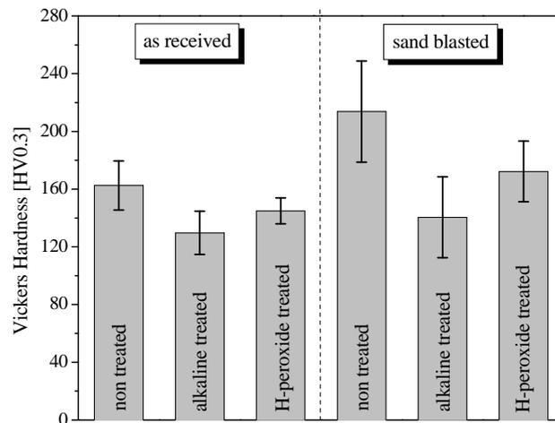
Fig. 6. Hardness values of surface for the chemically treated and non-treated specimens.
