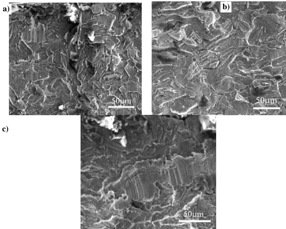
Fig. 8. Fracture cross sections of the chemically treated and non treated samples. (a) non-treated, (b) alkaline treated, (c) peroxide treated.
