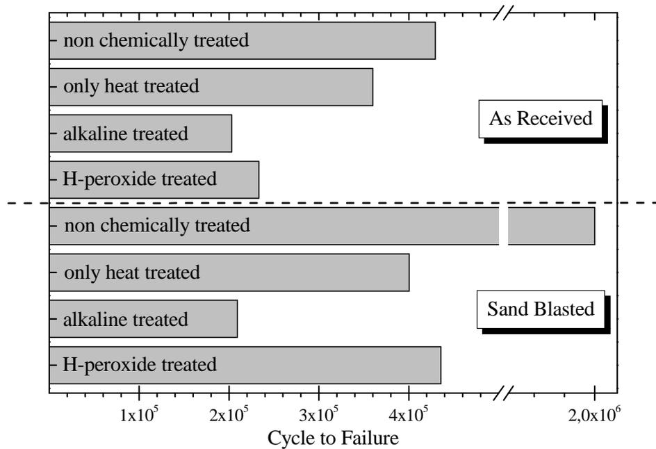
Fig. 7. Cycle to failure values for the chemically treated and non-treated specimens.
