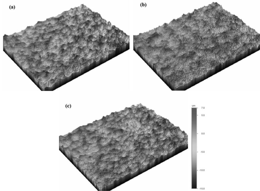
Fig. 5. Surface topographies of the sand blasted samples a) chemically non-treated, b) alkaline treated, c) hydrogen peroxide treated.
