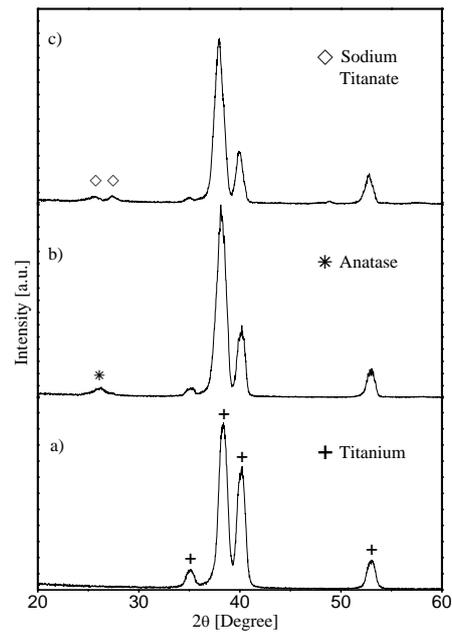
Fig. 2 X-Ray pattern of the as-received samples; (a) non-treated, (b) hydrogen-peroxide-treated and (c) alkaline-treated.
