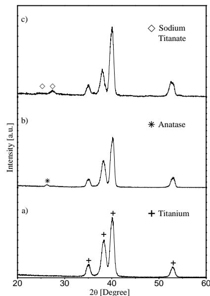
Fig. 3. X-Ray pattern of the sand blasted samples; (a) non-treated, (b) hydrogen-peroxide-treated and (c) alkaline-treated.
