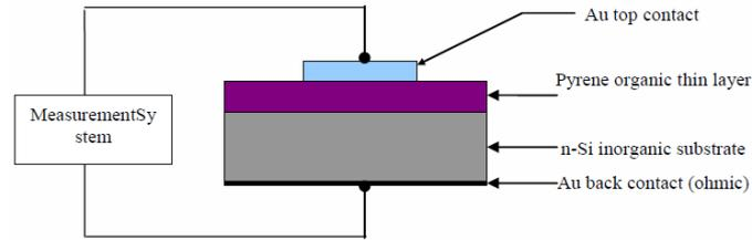
Fig. 2. The components of the Au/Pyrene/*n*-Si organic/inorganic semiconductor device for the electrical characterization
