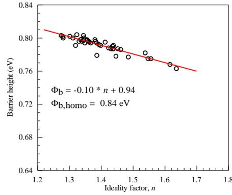
Fig. 7. The Barrier height vs. ideality factor plot obtained from the forward bias  $I$ - $V$  characteristics of the Au/Pyrene/ $n$ -Si organic/inorganic semiconductor device
