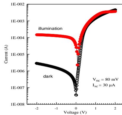
Fig. 16. (Color online) Current-Voltage characteristics of one of the Au/Pyrene/n-Si organic/inorganic semiconductor devices in dark and under light illumination.
