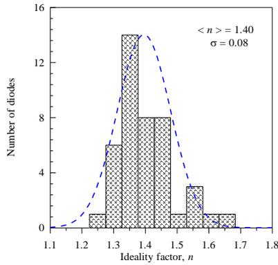
Fig. 5. The Gaussian distribution of ideality factors from the forward bias I-V characteristics of the Au/Pyrene/n-Si organic/inorganic semiconductor device
