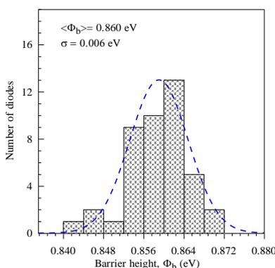
Fig. 9. The Gaussian distribution of the barrier heights from the Norde functions ( $F$ - $V$ ) of the Au/Pyrene/ $n$ -Si organic/inorganic semiconductor device
