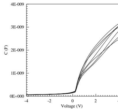
Fig. 11. Capacitance-Voltage characteristics of the selected seven Au/Pyrene/n-Si organic/inorganic semiconductor devices
