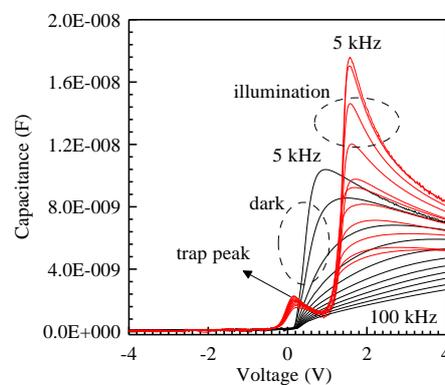
Fig. 17. (Color online) Capacitance-Voltage characteristics of the one of the Au/Pyrene/n-Si organic/inorganic semiconductor devices for various frequencies in dark and under light illumination. (Black lines are in dark, red lines are under light illumination)
