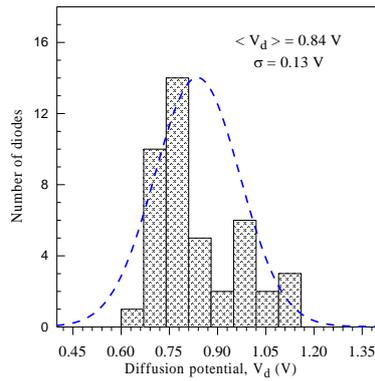
Fig. 14. The Gaussian distribution of the diffusion potential from the reverse bias  $C^2$ - $V$  characteristics of the Au/Pyrene/ $n$ -Si organic/inorganic semiconductor device
