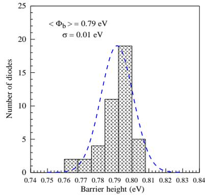
Fig. 4. The Gaussian distribution of barrier heights from the forward bias I-V characteristics of the Au/Pyrene/n-Si organic/inorganic semiconductor device.
