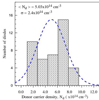
Fig. 15. The Gaussian distribution of the donor carrier concentrations from the reverse bias  $C^2$ - $V$  characteristics of the Au/Pyrene/ $n$ -Si organic/inorganic semiconductor device
