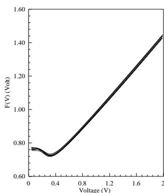
Fig. 8. Norde  $F(V)$ - $V$  characteristics of the selected seven Au/Pyrene/ $n$ -Si organic/inorganic semiconductor devices
