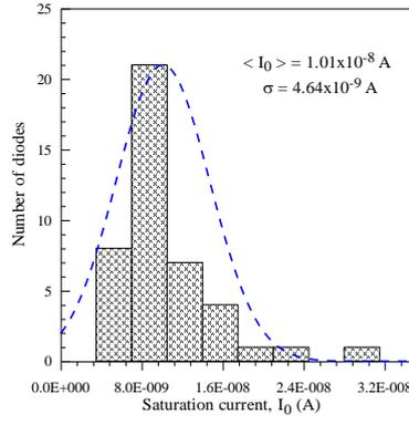
Fig. 6. The Gaussian distribution of saturation currents from the forward bias  $I$ - $V$  characteristics of the Au/Pyrene/ $n$ -Si organic/inorganic semiconductor device
