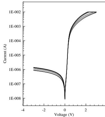
Fig. 3. Current-Voltage characteristics of the selected seven Au/Pyrene/*n*-Si organic/inorganic semiconductor devices
