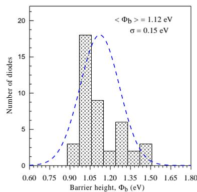
Fig. 13. The Gaussian distribution of barrier heights from the reverse bias  $C^2$ - $V$  characteristics of the Au/Pyrene/n-Si organic/inorganic semiconductor device
