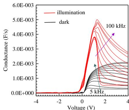
Fig. 18. (Color online) Conductance-Voltage characteristics of the one of the Au/Pyrene/n-Si organic/inorganic semiconductor devices for various frequencies in dark and under light illumination. (Black lines are in dark, red lines are under light illumination)
