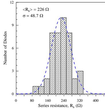
Fig. 10. The Gaussian distribution of the series resistances from the Norde functions ( $F$ - $V$ ) of the Au/Pyrene/ $n$ -Si organic/inorganic semiconductor device
