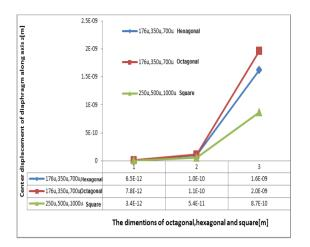
Fig.3: Comparison of the average center displacement of the Octagonal diaphragm with Hexagonal and Square diaphragms in term of frequency range (20Hz-20 kHz).
