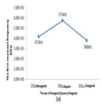
Fig. 4: Comparing the resonant frequency of Octagonal, Square and Hexagonal diaphragms.
