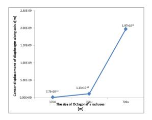
*Fig. 2: comparison of the average center displacement of the octagonal diaphragm with a radius of 176 μm, 350 μm and 700 μm in term of frequency range (20 Hz-20 kHz).*
