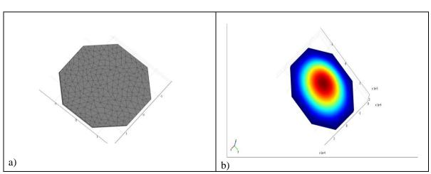
Mesh analysis and 3D simulation of the proposed diaphragm have been shown in Fig. (1-a , 1-b).
