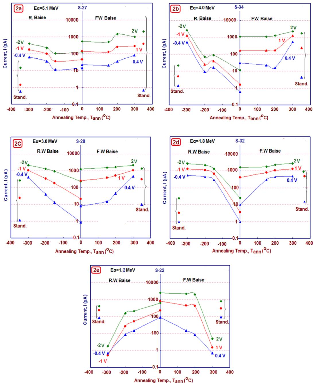
Fig. 2. Shows how current changes with annealing temperature in devices hit with alpha particles of varied energy 0.4, 1, and 2 V.
