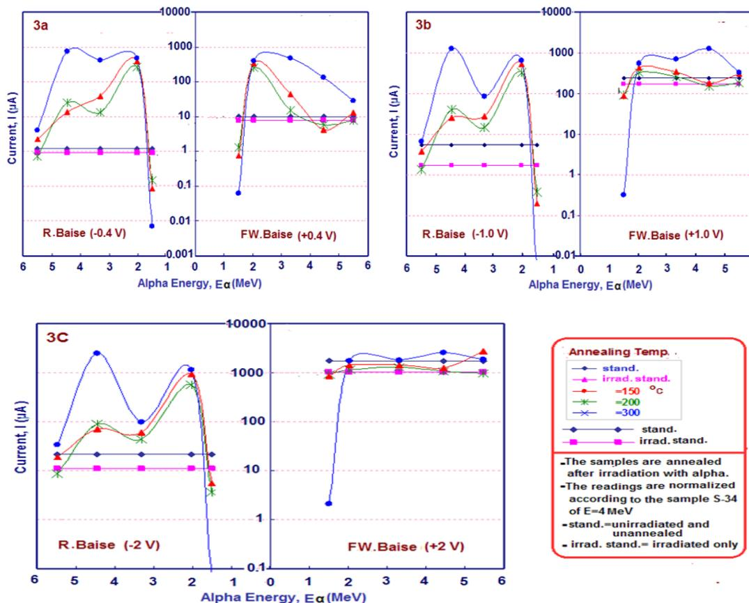
Fig. 3. Current versus alpha-particle-energy variation at different annealing temperatures and reverse bias voltages.
