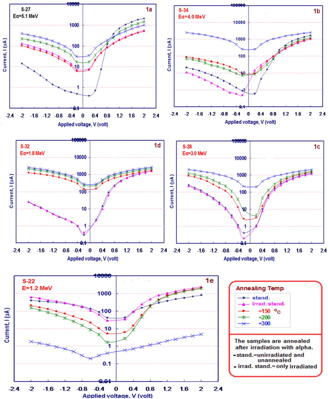
Fig. 1. The I-V characteristics of annealed devices after being irradiated with various energy of alpha particles.
