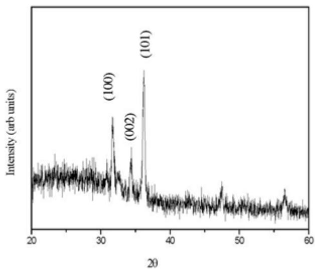
Fig.1: XRD pattern of ZnO thin film annealed at 350 °C
