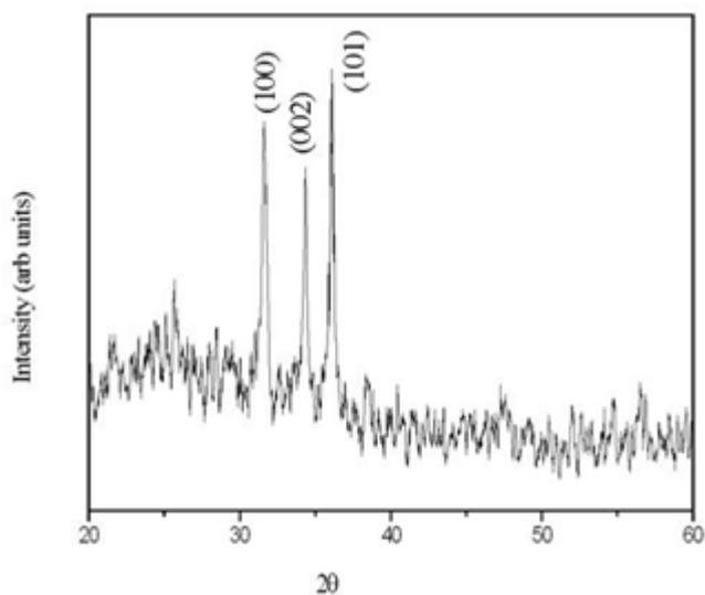
Fig.3: XRD pattern of ZnO thin film annealed at 450 °C
