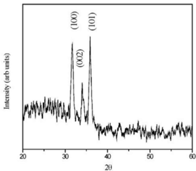
Fig.2: XRD pattern of ZnO thin film annealed at 400 °C
