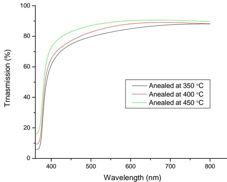
Fig. 5: Transmission spectra of ZnO thin films at different temperature.
