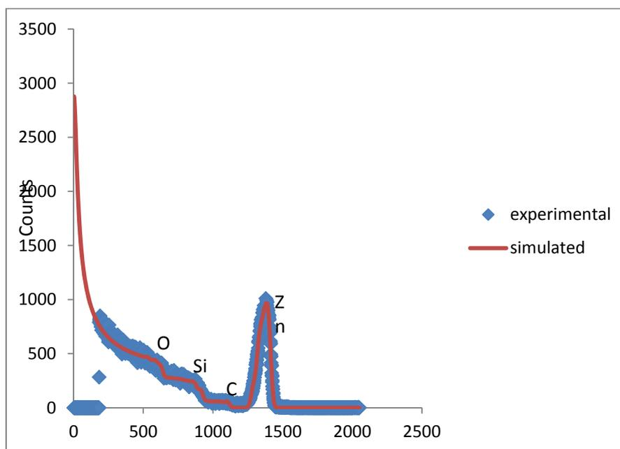
Fig. RBS spectrum for zinc oxide thin film annealed at 450 °C
