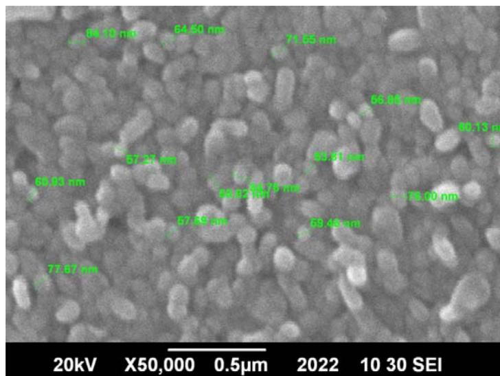
Fig.4: SEM micrographs of ZnO thin film annealed (a) at 350 °C, (b) at 450 °C
