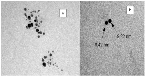
Fig. (1).TEM image of spherical silver nanoparticles
