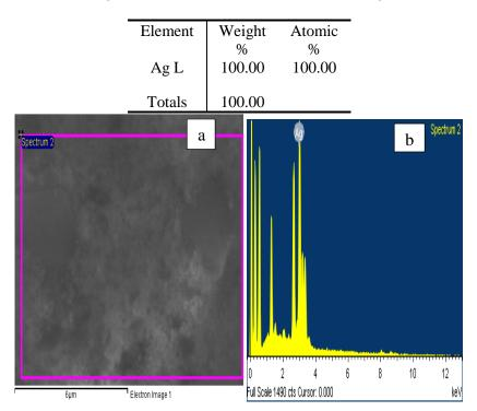
Fig2. (a) SEM image, (b) EDS pattern of spherical AgNPs prepared. Table .EDS elemental micro-analysis of the AgNPs
