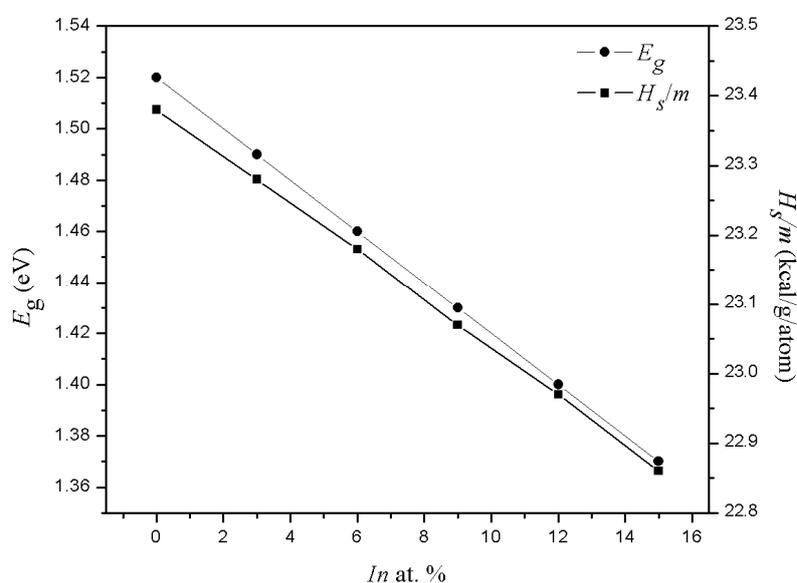
Fig. 3: Plot of  $E_g$  and  $H_s/m$  against increasing  $In$  at. % in  $Sb_{10}Se_{65}Ge_{25-y}In_y$  ( $y = 0, 3, 6, 9, 12, 15$ ) glass system.
