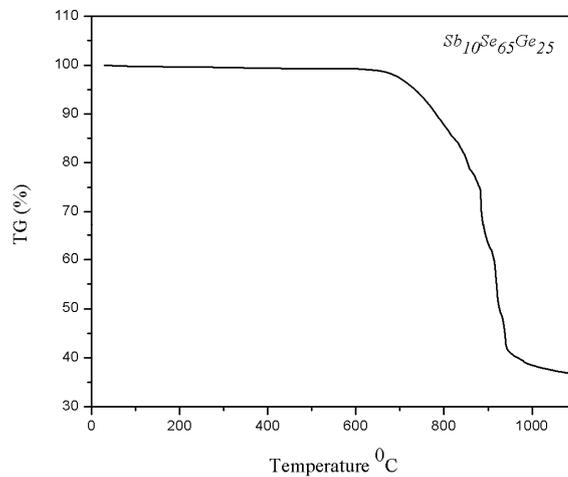
Fig. 1: Thermo Gravimetric (TG) %age variation with temperature for  $Sb_{10}Se_{65}Ge_{25}$  at heating rate of 10 °C/min.
