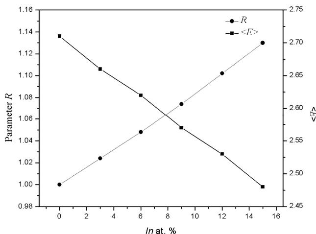
Fig. 2: Variation of Parameter  $R$  and mean bond energy ( $\langle E \rangle$ ) with increasing  $In$  content in  $Sb_{10}Se_{65}Ge_{25-y}In_y$  ( $y = 0, 3, 6, 9, 12, 15$ ) glass system.
