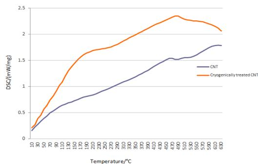
Fig 4 Thermogravimetric behavior of cryogenic treated and untreated MWCNTs for heat absorption
