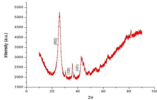
*Fig. 6. XRD pattern of untreated MWCNTs*
