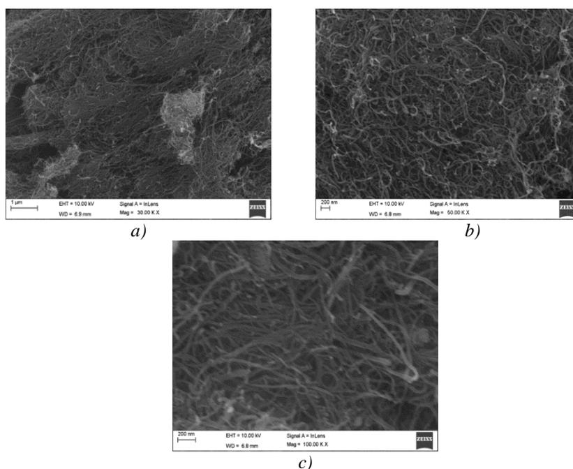
Fig. 2 SEM Image of cryogenic untreated MWCNTs with various magnification factor (a) 30KX, (b) 50KX, (c) 100KX
