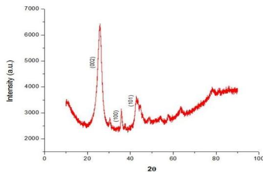
*Fig. 7. XRD pattern of cryogenically treated MWCNTs*
