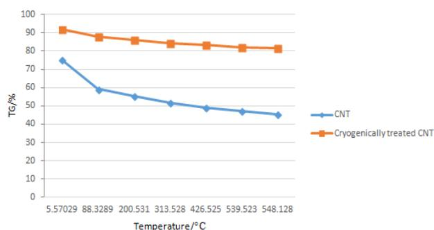
Fig 5 Thermogravimetric behavior of cryogenic treated and untreated MWCNTs for residual mass
