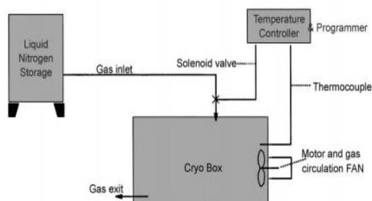
Fig. 1 Schematic illustration of the process of cryogenic treatment
