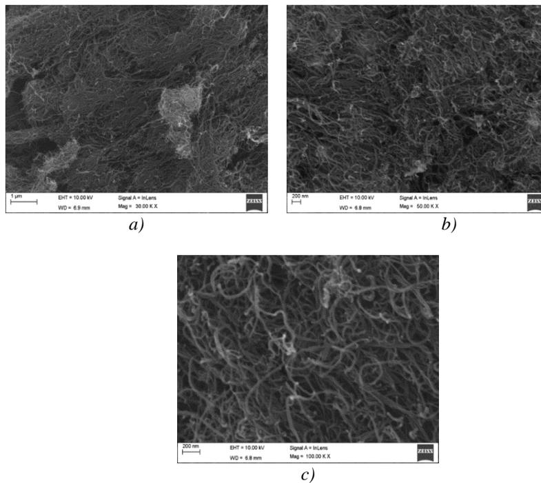
Fig. 3 SEM Image of cryogenic treated MWCNTs with various magnification factor (a) 30KX, (b) 50KX, (c) 100KX
