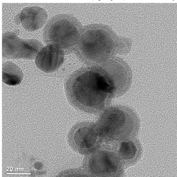
Fig.2. TEM images of carbon coated iron nanoparticles
