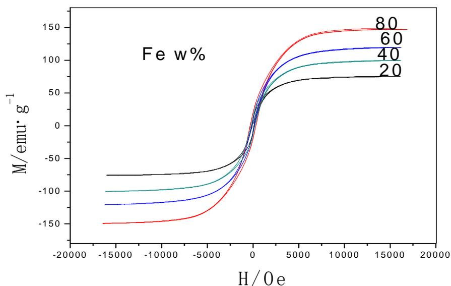
Fig.3. Magnetic field dependence of magnetization of different content iron carbon coated
