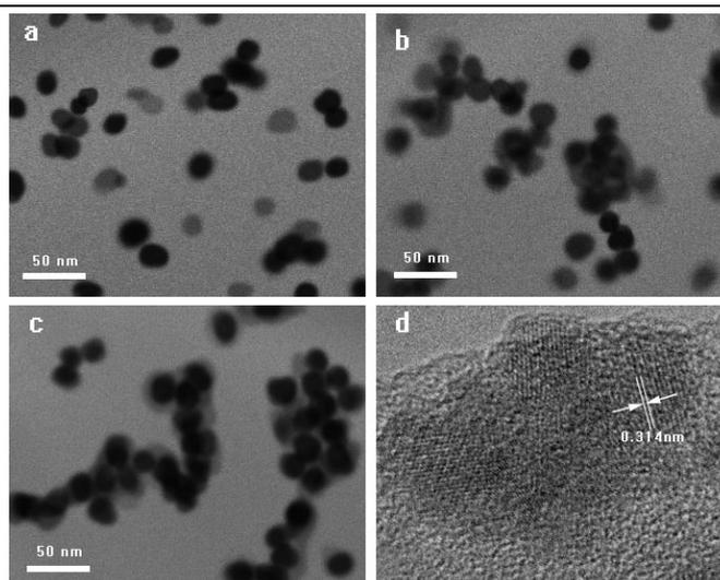
Fig. 3 TEM images of (a) undoped ZnS; (b) 1% Ag doped ZnS nanoparticles; (c) 2% Ag doped ZnS nanoparticles; (d) HRTEM image of 2% Ag doped ZnS nanoparticles
