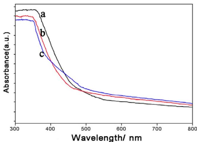
Fig. 5 UV-vis spectra of (a) undoped ZnS; (b) 1% Ag doped ZnS nanoparticles; (c) 2% Ag doped ZnS nanoparticles.
