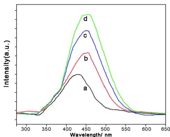
Fig. 6 PL spectra of (a) undoped ZnS; (b) 0.5% Ag doped ZnS nanoparticles; (c) 1% Ag doped ZnS nanoparticles; (d) 2% Ag doped ZnS nanoparticles.
