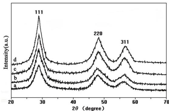
Fig. 1 XRD patterns of undoped ZnS (a) and Ag-doped ZnS nanocrystals (b: 0.5%; c: 1%; d: 2%)
