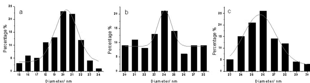
Fig. 4 Size distribution of (a) undoped ZnS; (b) 1% Ag doped ZnS nanoparticles; (c) 2% Ag doped ZnS nanoparticles.
