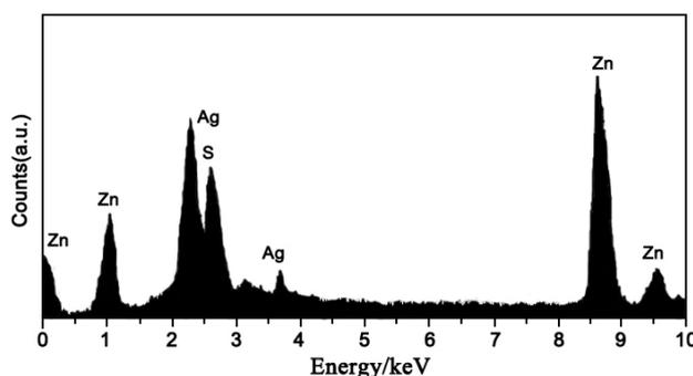
Fig. 2 EDX spectrum of as prepared Ag-doped ZnS nanocrystals.
