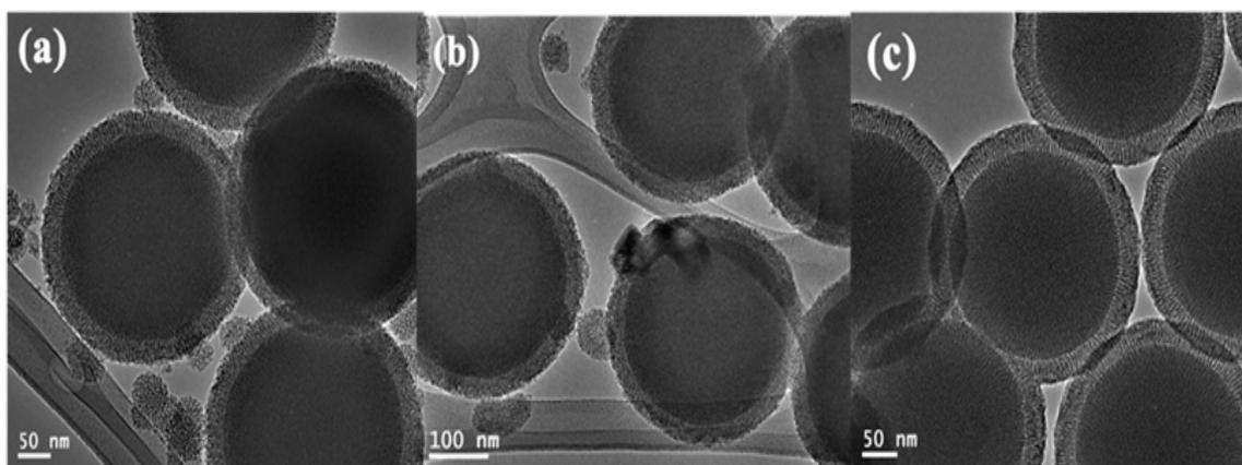
Fig. 2. TEM images of double mesoporous core-shell silica nanospheres with different BET surface area of (a) 129.8, (b) 137.9, and (c) 148.9 cm<sup>2</sup>/g.
