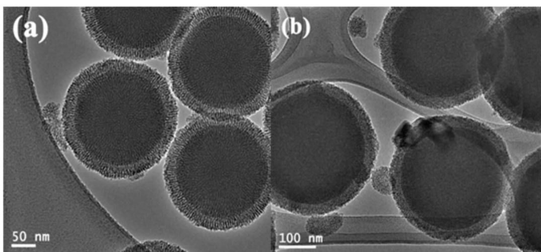
Fig. 6. TEM images of double mesoporous core-shell silica nanospheres with different pore volume of (a) 5 nm, and (b) 3.9 nm.
