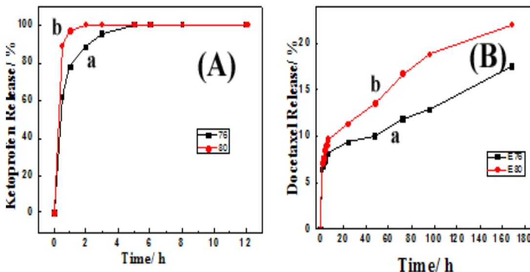
Fig. 7. In-vitro release study of (A) ketoprofen and (B) docetaxel loaded within double mesoporous core-shell silica spheres with different with different pore volume of (a) 5 nm, and (b) 3.9 nm.
