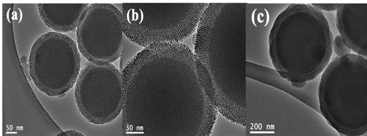
Fig. 4. TEM images of double mesoporous core-shell silica nanospheres with different shell thickness (a) 28 nm, (b) 45 nm, (c) 55 nm and total pore volume of (a) 0.301, (b) 0.343, and (c) 0.371 cc/g.
