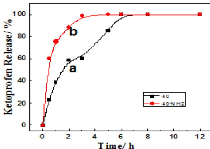
Fig. 8. In-vitro release study of ketoprofen loaded within double mesoporous core-shell silica spheres with (a) no functionalization, and (b) amino-functionalization.
