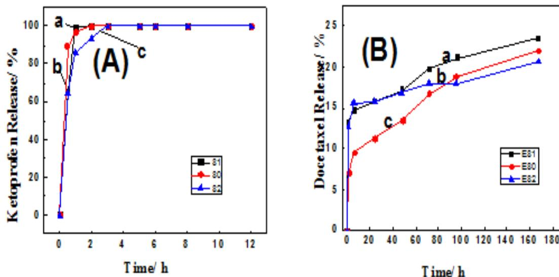
Fig. 3. In-vitro release study of (A) ketoprofen and (B) docetaxel loaded within double mesoporous core-shell silica spheres with different BET surface area of (a) 129.8, (b) 137.9, and (c) 148.9  $\text{cm}^2/\text{g}$ .
