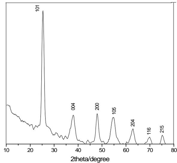
*Fig. 1. XRD Pattern of TiO<sub>2</sub> nanoparticles*
