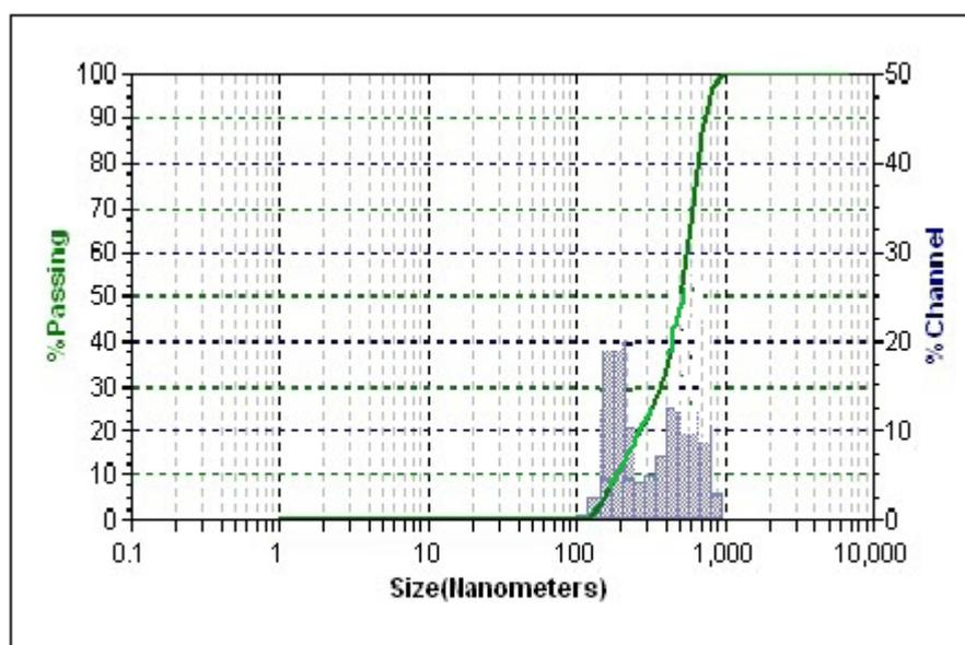
Fig. 3. Particle size distribution of  $\text{TiO}_2$  nanoparticles
