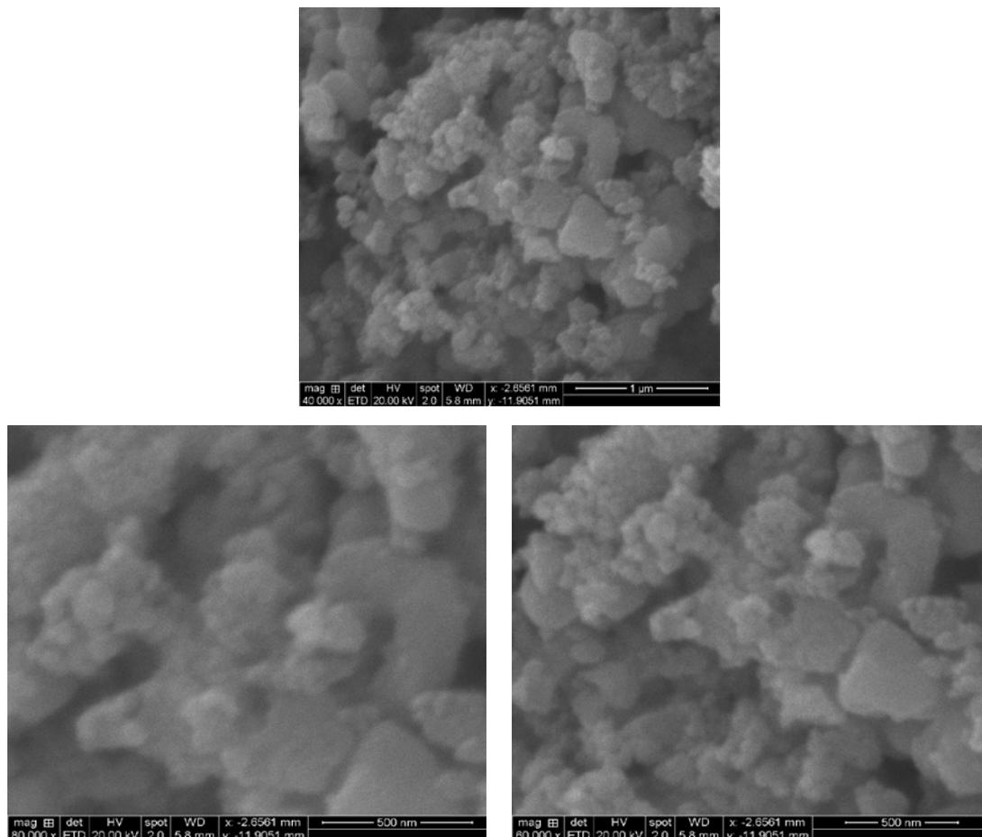
*Fig. 2. SEM micrographs of TiO<sub>2</sub> nanoparticles*
