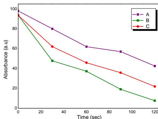
Fig. 5.3. Photocatalytic degradation of MO over the ZnMgTiO<sub>2</sub> nanocomposites (A) Zn<sub>0.08</sub>Mg<sub>0.01</sub>TiO<sub>0.01</sub>, (B) Zn<sub>0.08</sub>Mg<sub>0.005</sub>TiO<sub>0.015</sub>, (C) Zn<sub>0.08</sub>Mg<sub>0.015</sub>TiO<sub>0.005</sub>
