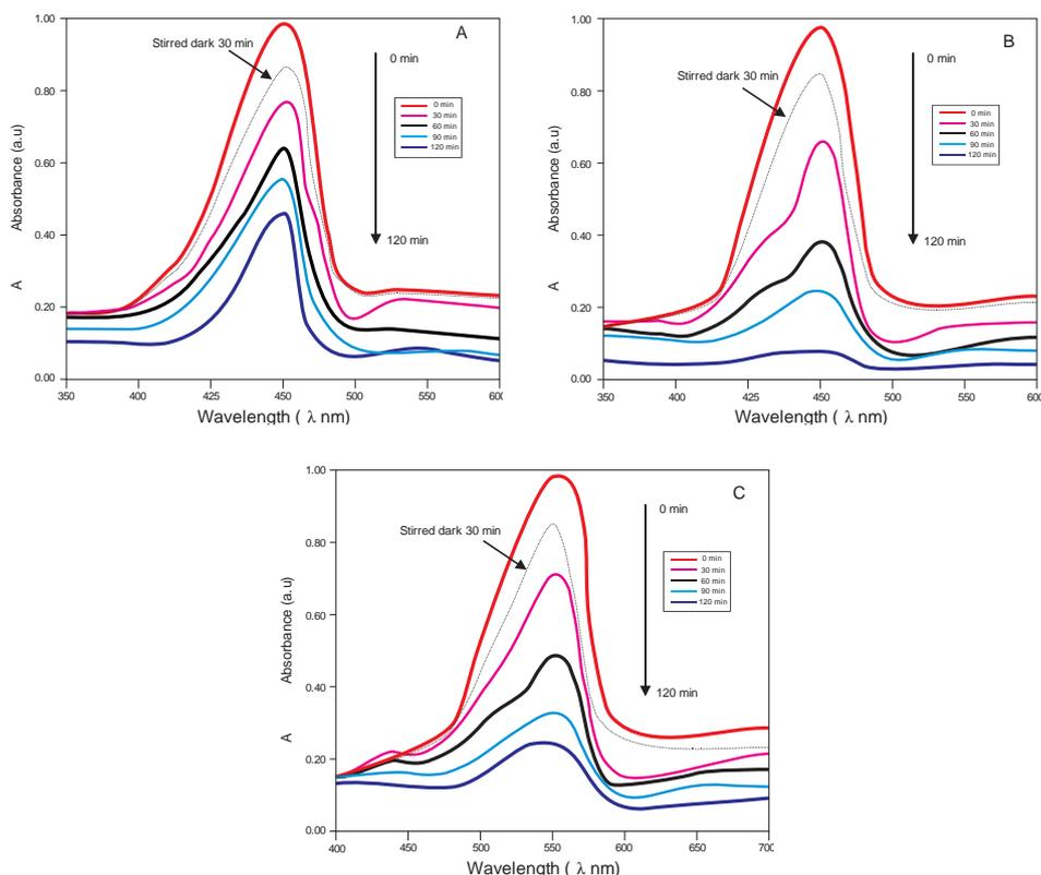
Fig. 5.1. UV-Vis absorption spectra of ZnMgTiO<sub>2</sub> nanocomposites (A) Zn<sub>0.08</sub>Mg<sub>0.01</sub>TiO<sub>0.01</sub>, (B) Zn<sub>0.08</sub>Mg<sub>0.005</sub>TiO<sub>0.015</sub>, (C) Zn<sub>0.08</sub>Mg<sub>0.015</sub>TiO<sub>0.005</sub>.
