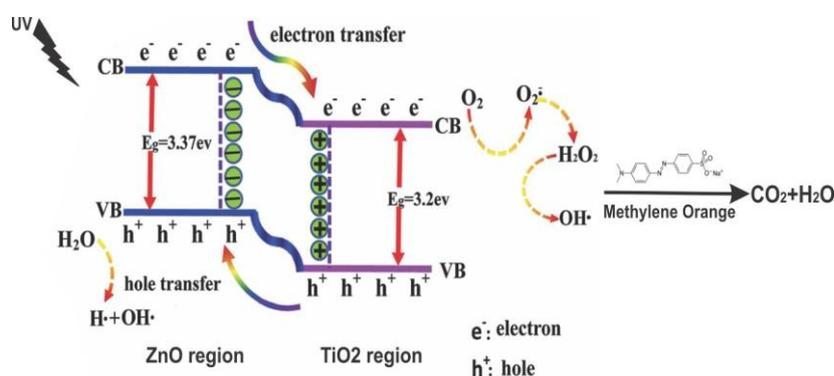
Fig. 5.2. Structure of the  $\text{ZnO-TiO}_2$  junction.
