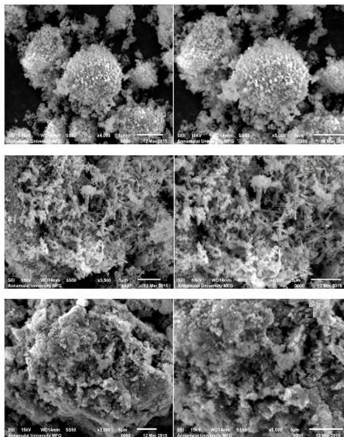
*Fig. 4. SEM morphological images of  $\text{Zn}_{0.08}\text{Mg}_{0.01}\text{TiO}_{0.01}$ ,  $\text{Zn}_{0.08}\text{Mg}_{0.005}\text{TiO}_{0.015}$ , &  $\text{Zn}_{0.08}\text{Mg}_{0.015}\text{TiO}_{0.005}$  nanocomposite.*
