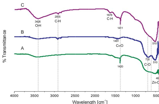
Fig. 2. FTIR spectra of nanocomposites (A)  $\text{Zn}_{0.08}\text{Mg}_{0.01}\text{TiO}_{0.01}$ , (B)  $\text{Zn}_{0.08}\text{Mg}_{0.005}\text{TiO}_{0.015}$ , (C)  $\text{Zn}_{0.08}\text{Mg}_{0.015}\text{TiO}_{0.005}$
