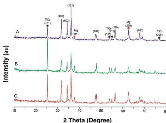
Fig. 1. XRD spectra of ZnMgTiO<sub>2</sub> nanocomposites (A) Zn<sub>0.08</sub>Mg<sub>0.01</sub>TiO<sub>0.01</sub>, (B) Zn<sub>0.08</sub>Mg<sub>0.005</sub>TiO<sub>0.015</sub>, (C) Zn<sub>0.08</sub>Mg<sub>0.015</sub>TiO<sub>0.005</sub>.
