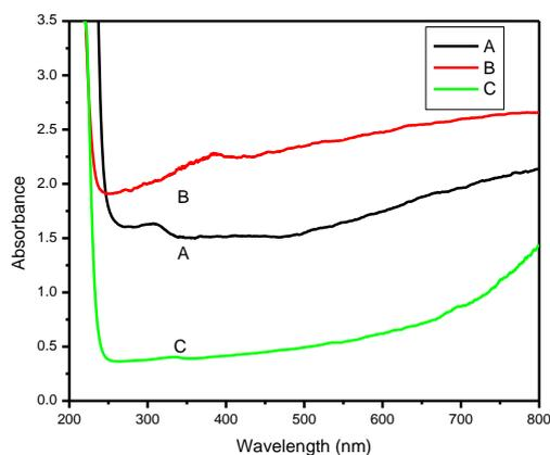
Fig. 3. UV-Visible spectra of  $\text{ZnMgTiO}_2$  nanocomposites (A)  $\text{Zn}_{0.08}\text{Mg}_{0.01}\text{TiO}_{0.01}$ , (B)  $\text{Zn}_{0.08}\text{Mg}_{0.005}\text{TiO}_{0.015}$ , (C)  $\text{Zn}_{0.08}\text{Mg}_{0.015}\text{TiO}_{0.005}$ .
