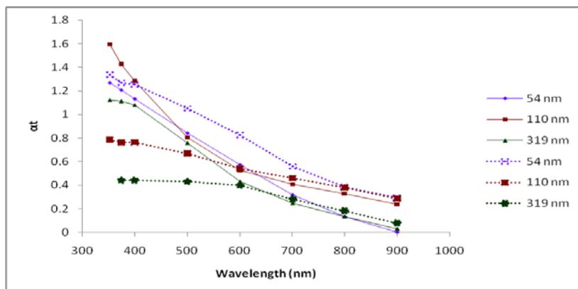
Fig. 5. Variation of optical density of as-deposited (solid line) and annealed (dotted line)  $(\text{Bi}_{0.95}\text{Sb}_{0.05})_2\text{S}_3$  films
