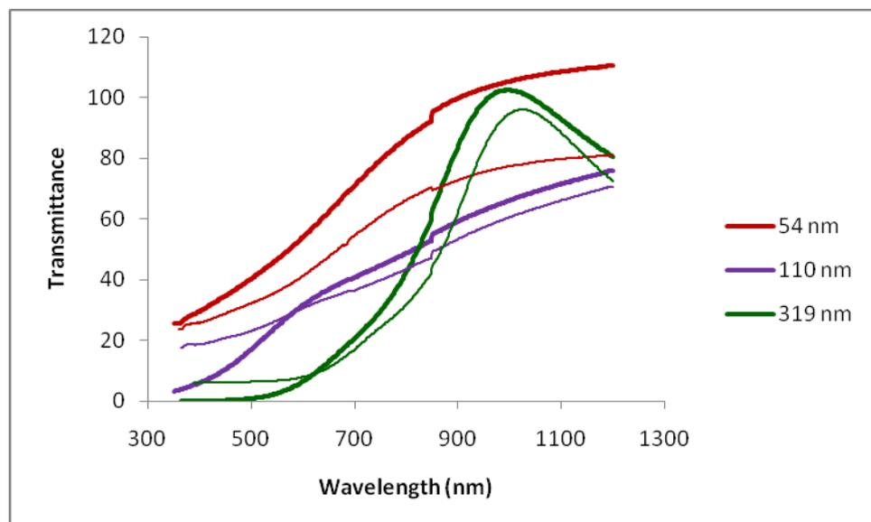
Fig. 4. Transmittance spectra of as-deposited (wide line) and annealed (narrow line) (Bi<sub>0.95</sub>Sb<sub>0.05</sub>)<sub>2</sub>S<sub>3</sub> films
