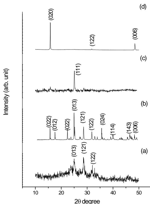
Fig. 1. XRD pattern of (a) Bi<sub>2</sub>S<sub>3</sub> thin film (b) (Bi<sub>0.95</sub>Sb<sub>0.05</sub>)<sub>2</sub>S<sub>3</sub> powder (c) as-deposited (Bi<sub>0.95</sub>Sb<sub>0.05</sub>)<sub>2</sub>S<sub>3</sub> thin film (d) annealed (Bi<sub>0.95</sub>Sb<sub>0.05</sub>)<sub>2</sub>S<sub>3</sub> thin film
