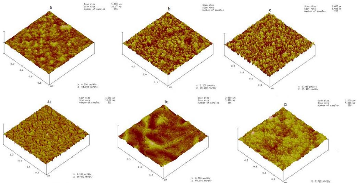
Fig. 3. Atomic force micrographs of as-deposited (a,b,c) and annealed (a<sub>1</sub>,b<sub>1</sub>,c<sub>1</sub>) (Bi<sub>0.95</sub>Sb<sub>0.05</sub>)<sub>2</sub>S<sub>3</sub> films of thickness 54 nm, 110 nm, 319 nm
