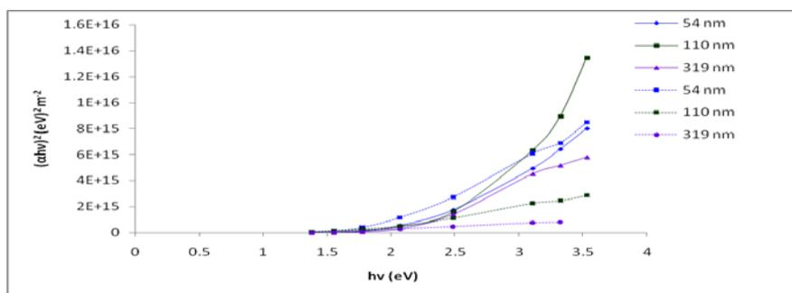
Fig. 6.  $(\alpha h\nu)^2$  Vs.  $h\nu$  plot of as-deposited and annealed  $(\text{Bi}_2\text{S}_3)_{0.95}(\text{Sb}_2\text{S}_3)_{0.05}$  films
