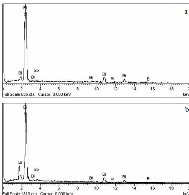
Fig. 2. EDAX spectrum of (a)  $(\text{Bi}_{0.95}\text{Sb}_{0.05})_2\text{S}_3$  powder (b)  $(\text{Bi}_{0.95}\text{Sb}_{0.05})_2\text{S}_3$  thin film
