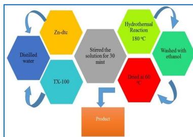
Fig. 2 Reaction scheme of ZnS.
