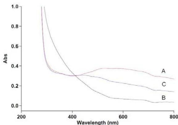
Fig. 3. UV - Vis spectra of  $\beta\text{-In}_2\text{S}_3$  nanoparticles prepared from (A)  $\text{In}(\text{NO}_3)_3 \cdot x\text{H}_2\text{O}$ , (B)  $\text{InCl}_3$  and (C)  $\text{In}_2(\text{SO}_4)_3$
