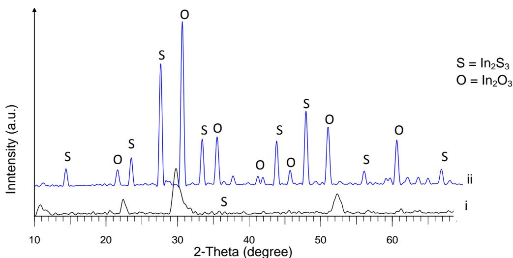
Fig. 1b. XRD patterns of the product prepared with  $\text{In}(\text{CH}_3\text{COO})_3$  before (i) and after (ii) heating to 773 K
