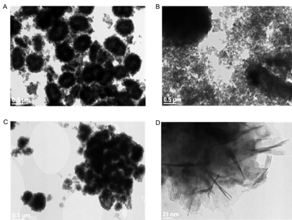
Fig. 2. TEM images of  $\beta$ - $\text{In}_2\text{S}_3$  nanoparticles obtained with diverse indium source: (A)  $\text{In}(\text{NO}_3)_3 \cdot x\text{H}_2\text{O}$ , (B)  $\text{InCl}_3$  and (C)  $\text{In}_2(\text{SO}_4)_3$ , and (D) primary nanoparticles
