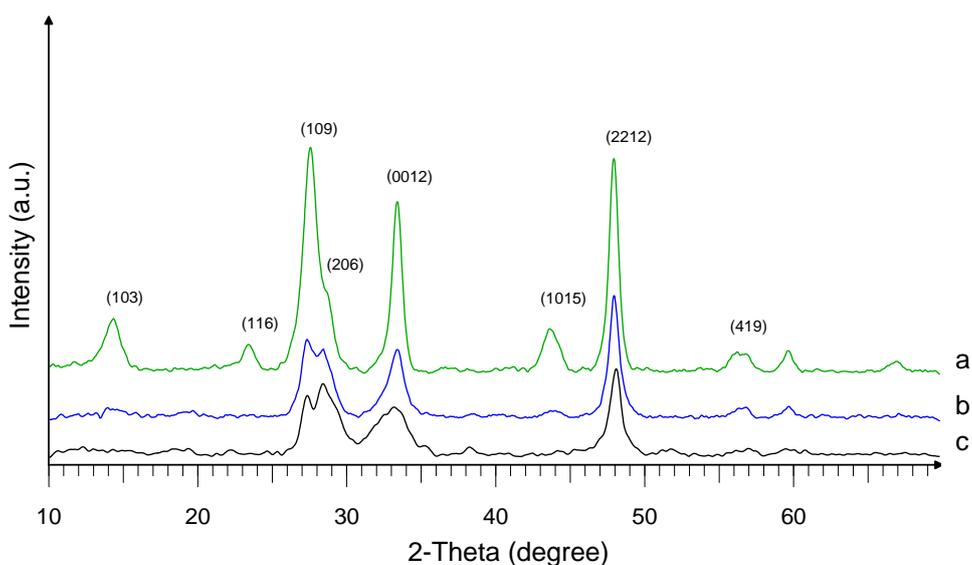
Fig. 1a. XRD patterns of the products prepared with (a)  $\text{In}(\text{NO}_3)_3 \cdot x\text{H}_2\text{O}$ , (b)  $\text{InCl}_3$  and (c)  $\text{In}_2(\text{SO}_4)_3$
