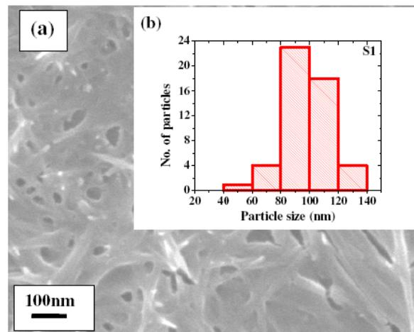
Fig. 1. Scanning Electron Microscope (SEM) image of the sample S1 is shown in (a) and the corresponding particle size distribution is shown in (b).
