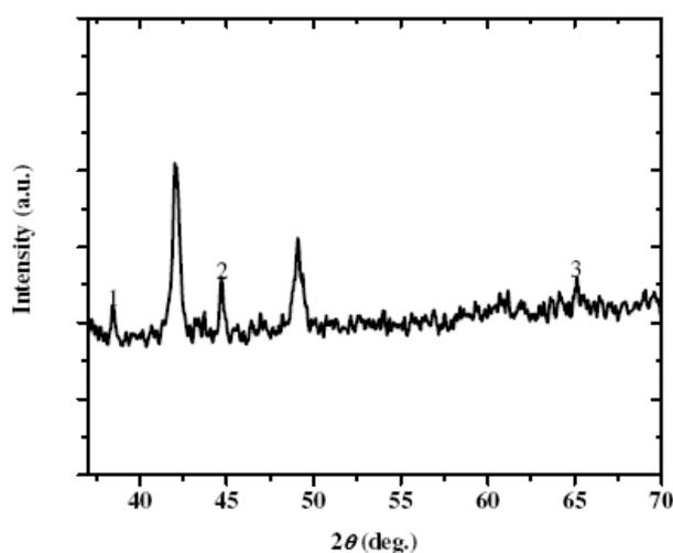
Fig. 4. Typical X-ray diffraction (XRD) pattern of the as-prepared silver nanoparticles, viz. for S2 sample. XRD peaks 1, 2, and 3 appear at  $38.1^{\circ}$ ,  $44.6^{\circ}$ , and  $64.8^{\circ}$  due to reflections from (111), (200), and (220) planes of silver (JCPDF: 03-0931), respectively.
