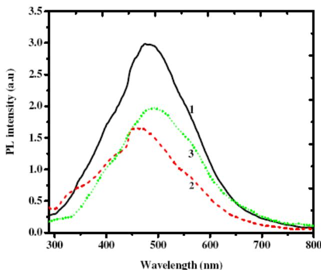
Fig. 6. Photoluminescence emission spectra of the aqueous solutions of all the samples, measured at room temperature. Curves marked as 1, 2, and 3 correspond to S1, S2, and S3 samples, respectively.
