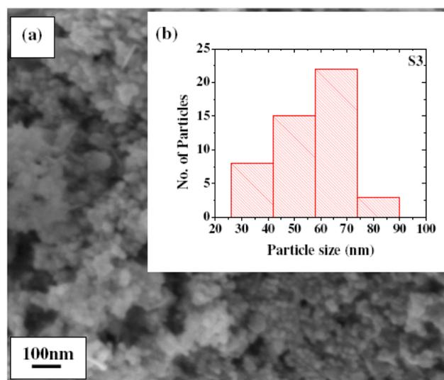
Fig. 3. Scanning Electron Microscope (SEM) image of the sample S3 is shown in (a) and the corresponding particle size distribution is shown in (b).
