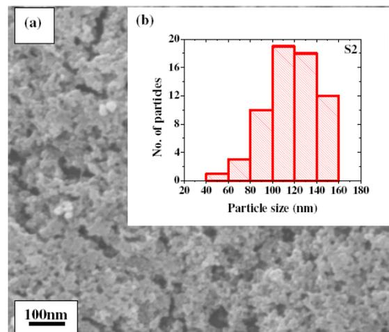
Fig. 2. Scanning Electron Microscope (SEM) image of the sample S2 is shown in (a) and the corresponding particle size distribution is shown in (b).
