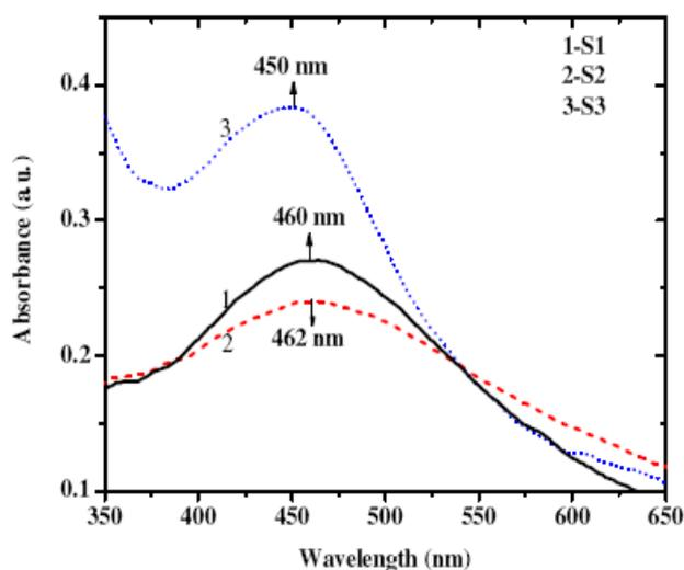
Fig. 5. UV-Visible absorption spectra of the aqueous solutions of all the samples, measured at room temperature. Curves marked as 1, 2, and 3 correspond to S1, S2, and S3 samples, respectively.
