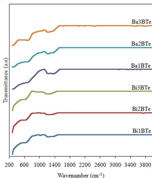
Fig. 2. FTIR spectra of all glass samples
