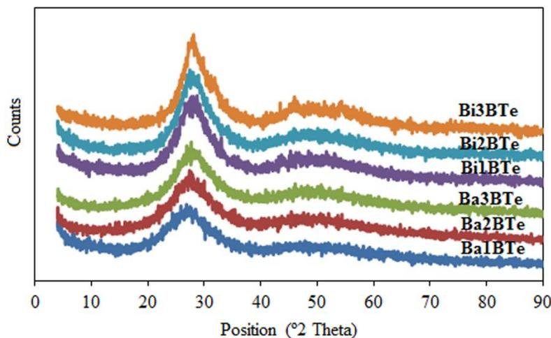
Fig 1. Diffractogram of the  $[(\text{TeO}_2)_{0.7}(\text{B}_2\text{O}_3)_{0.3}]_{1-x}(\text{Bi}_2\text{O}_3)_x$  and  $[(\text{TeO}_2)_{0.7}(\text{B}_2\text{O}_3)_{0.3}]_{1-x}(\text{BaO})_x$  glass systems
