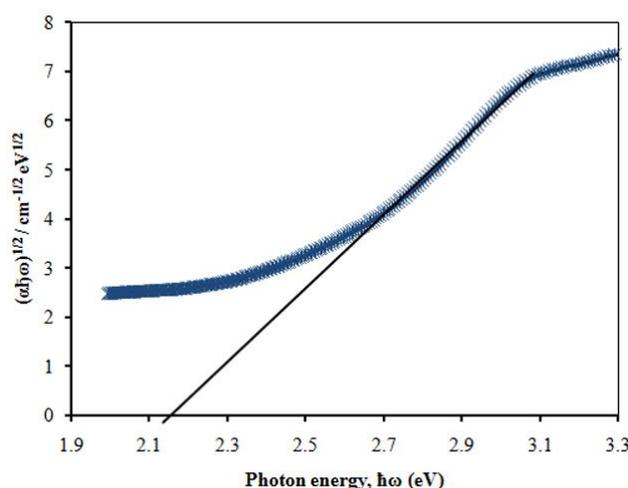
Fig. 3. Plot of  $\alpha\hbar\omega$  versus  $\hbar\omega$  for indirect transition of Bi3BTe glass.
