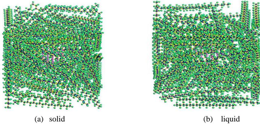
Fig. 6 The physical model of Al nanoparticles/octadecane composite phase change material
