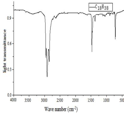
Fig. 9 C18H38 IR absorption spectra
