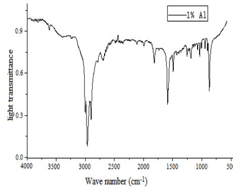
Fig. 10 IR absorption spectra of composite phase change materials
