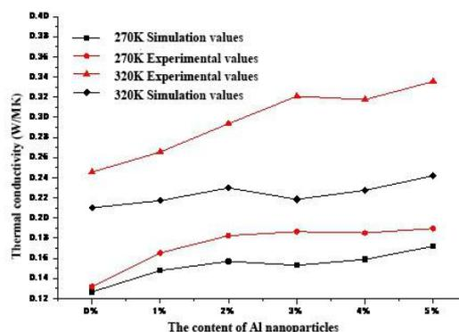
Fig. 12 Simulation and experimental values of composite phase change material thermal conductivity
