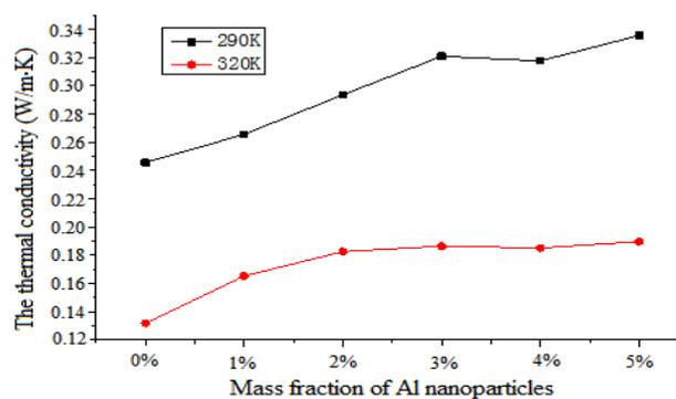
Fig. 11 Thermal conductivity of composite materials with different aluminum content
