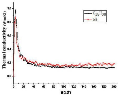
Fig. 7 Time history of the liquid PCM thermal conductivity
