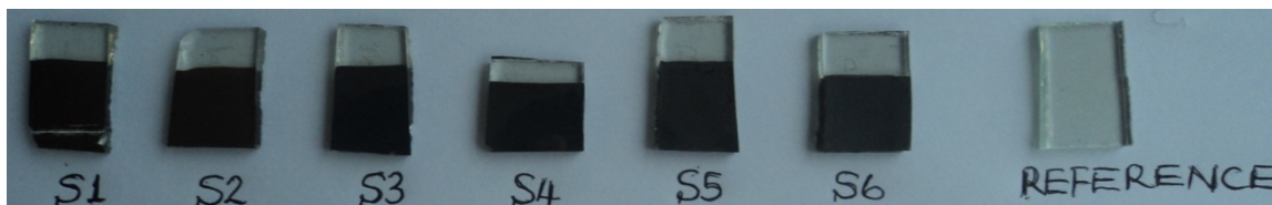
Fig. 3.1 Appearance of electro-deposited CdTe layers grown on glass FTO at different deposition times of 60,30,90,120,150 and 180 minutes for samples S1-S6 respectively.
