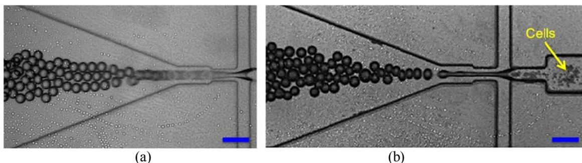
Fig. 2. Microdroplet generation in flow-focusing microfluidic channels using GelMa prepolymer solutions (a) without cells and (b) with cells; scale bar = 200  $\mu\text{m}$ .
