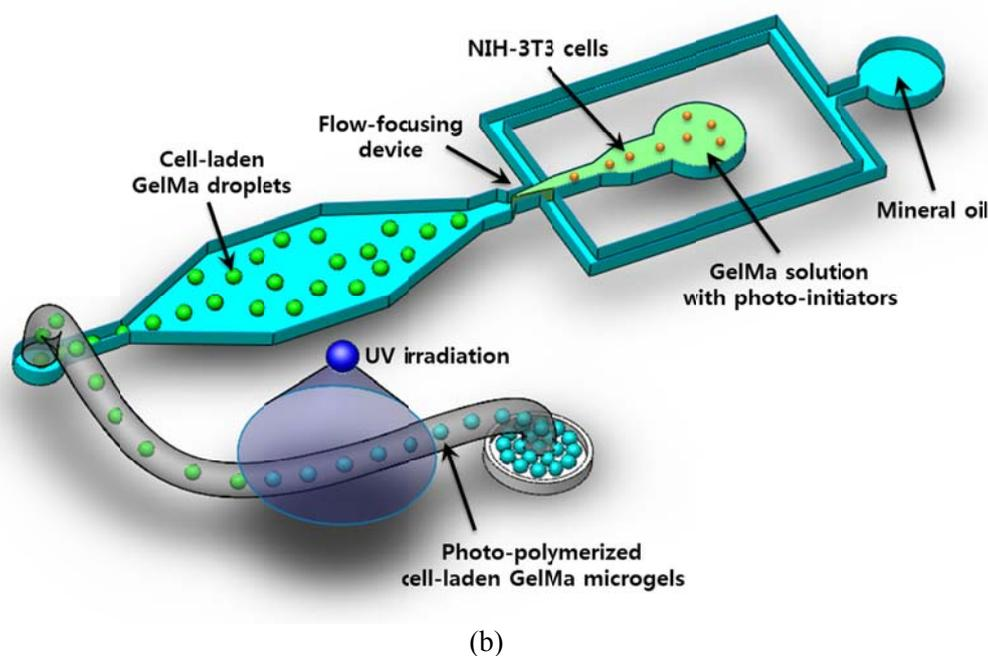
*Fig. 1. (a) Photo-polymerization reaction of GelMa driven by a photo-initiator; (b) schematic description of generation of photo-polymerized GelMa microgels in a flow-focusing microfluidic device. Flow-focusing channel width and height = 100  $\mu\text{m}$ .*
