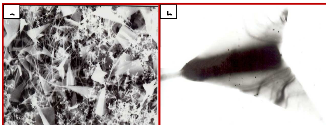
Fig. 7(a & b) low magnification and high magnification SEM image of the ZnO nanotetrapods-like network, respectively.
