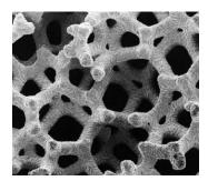
Fig. 2. Trabecular Metal (TM). An image made by scanning electron microscopy demonstrates highly porous microstructure.
