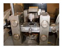
Fig. 4. General view of scratch tester with a diamond spherical segment.
