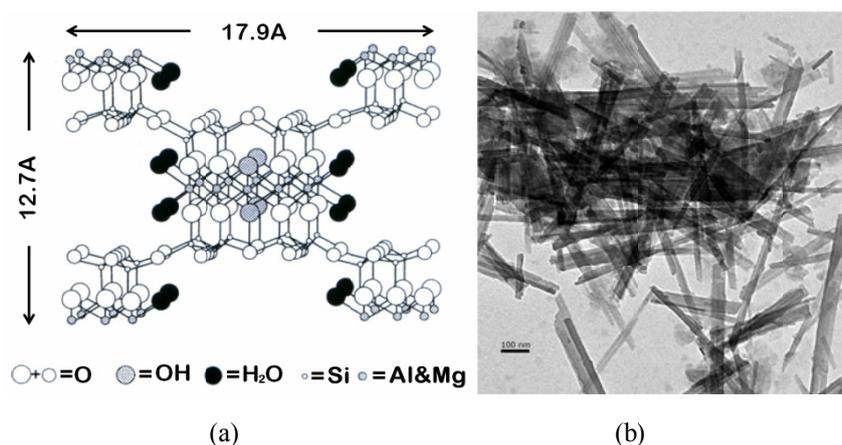
Fig. 1: (a) Crystal structure of attapulgite and (b) NATP TEM morphology.
