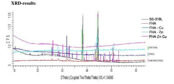
Fig 2.The compared diffractograme of FHA, and Cu and/or Zn dopped FHA
