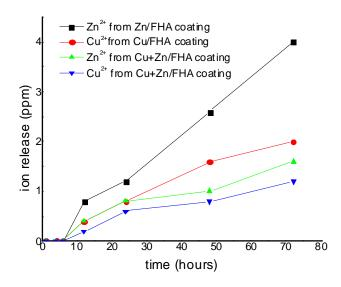
Fig.3. Evolution in time of ions release process
