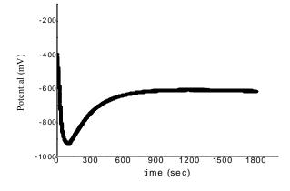
Fig1. The dependence potential versus time in the coating process SS 316L
