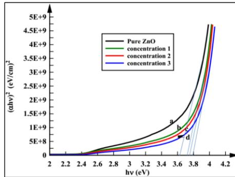
Fig. 7. Optical energy gap versus wavelength of nanocrystalline thin film: (a)- Undoped ZnO, (b)- ZnO:Al (0.05 M), (c)- ZnO:Al (0.10 M), (d)- ZnO:Al (0.15 M).
