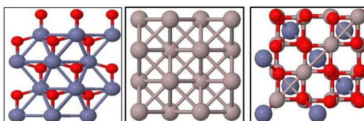
Fig. 2. Crystal structure of: (a)- Hexagonal ZnO, (b)- Aluminum and (c)- Aluminum doped zinc oxide (ZnO:Al)
