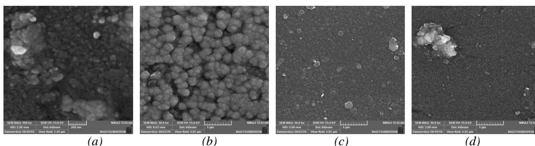
Fig. 3. SEM images of nanocrystalline thin film: (a)- Pure ZnO, (b)- ZnO:Al (0.05 M), (c)- ZnO:Al (0.10 M) (d)- ZnO:Al (0.15 M)
