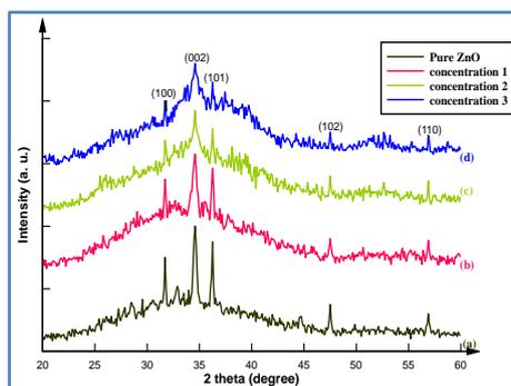
Fig. 1. XRD patterns of AZO thin films deposited with different aluminum concentrations (0.05, 0.10 and 0.15 M).
