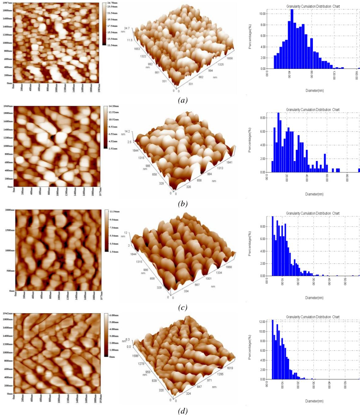
Fig. 4. AFM images of nanocrystalline thin film: (a)- Pure ZnO, (b)- ZnO:Al (0.05 M), (c)- ZnO:Al (0.10 M), (d)- ZnO:Al (0.15 M)
