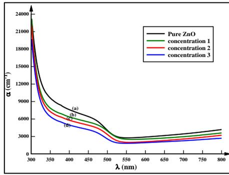
Fig. 6. Absorption coefficient versus wavelength of nanocrystalline thin film: (a)- Undoped ZnO, (b)- ZnO:Al (0.05 M), (c)- ZnO:Al (0.10 M), (d)- ZnO:Al (0.15 M)
