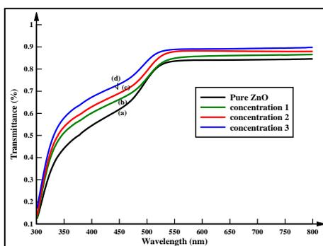
Fig. 5. Transmittance versus wavelength of nanocrystalline thin film: (a)- Undoped ZnO, (b)- ZnO:Al (0.05 M), (c)- ZnO:Al (0.10 M), (d)- ZnO:Al (0.15 M).
