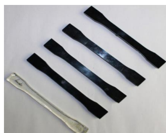
Fig.2: Dog bone shape pure epoxy and MWCNTs/alumina hybrid nanocomposites specimen after polishing
