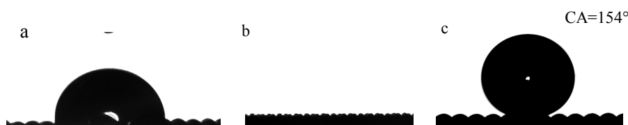
Fig. 8. The surface wetting illustration and the corresponding CA value of CM (a), OCM (b) and SOCM (c), respectively.
