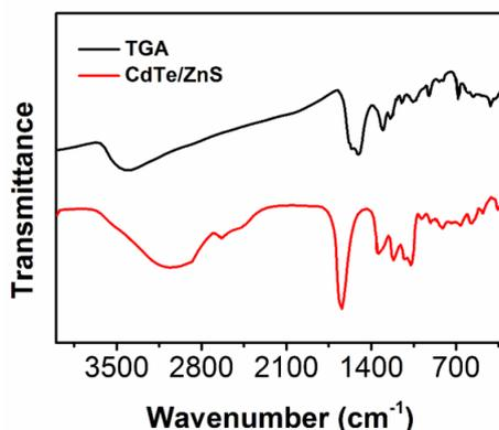
Fig. 3. FTIR spectra of TGA and CdTe/ZnS NPs.
