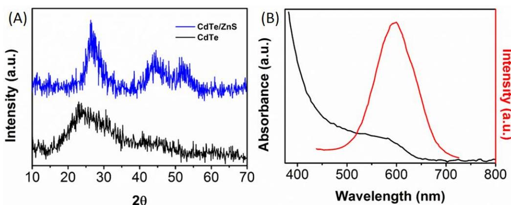
Fig. 2. (A) XRD patterns of CdTe NPs and CdTe/ZnS NPs. (B) UV-vis absorption spectrum and fluorescence emission spectrum of CdTe/ZnS NPs
