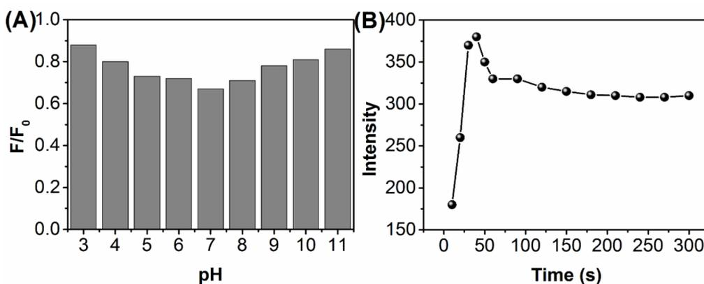
Fig. 4. (A) Effect of pH on the fluorescence intensity of CdTe/ZnS NPs. (B) Effect of reaction time on the fluorescence intensity of the CdTe/ZnS
