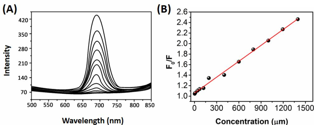
Fig. 5. (A) Fluorescence emission spectra of CdTe/ZnS NPs in the absence and presence of norfloxacin and presence of norfloxacin in concentrations of 5, 80, 200, 400, 600, 800, 1000, 1200, 1300 and 1400  $\mu\text{M}$ . (B) Linear curve of the relative fluorescence intensity ( $F_0/F$ ) versus the concentrations of norfloxacin.
