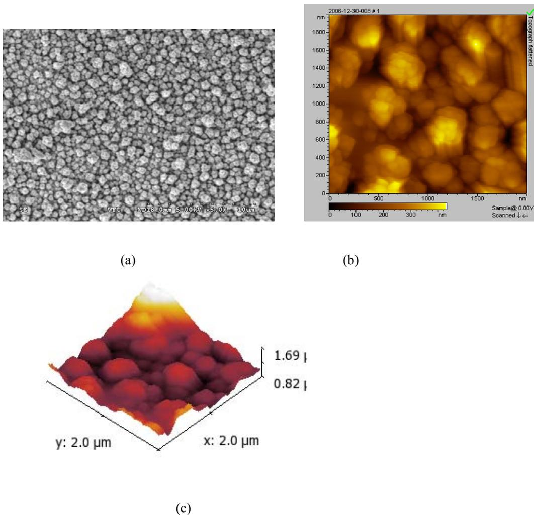
Fig. 5 (a) A high resolution SEM image, (b) 2D AFM image, and (c) 3D image of the  $\text{CuInSe}_2$  film with Cu, In, and Se close to the ratio of 1:1:2.
