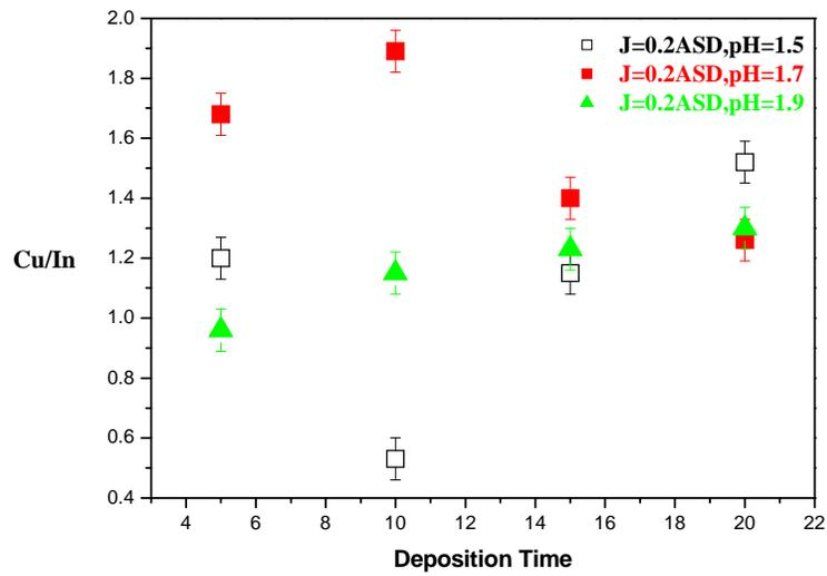
Fig. 3 The deposition time and the pH value versus Cu/In ratio in the  $\text{CuInSe}_2$  film.
