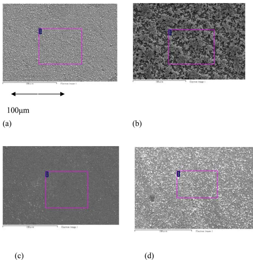
Fig. 1 Surface morphology of (a) Cu-rich film (b) In-rich film (c) Se-rich film (d) The  $\text{CuInSe}_2$  film with Cu, In, and Se ratio close to 1:1:2.
