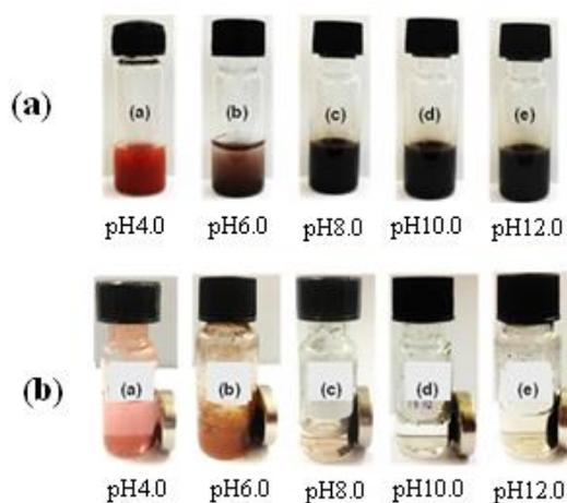
Fig.1 The prepared CoFe<sub>2</sub>O<sub>4</sub> suspension before (a) and after (b) application of the external magnetic field.
