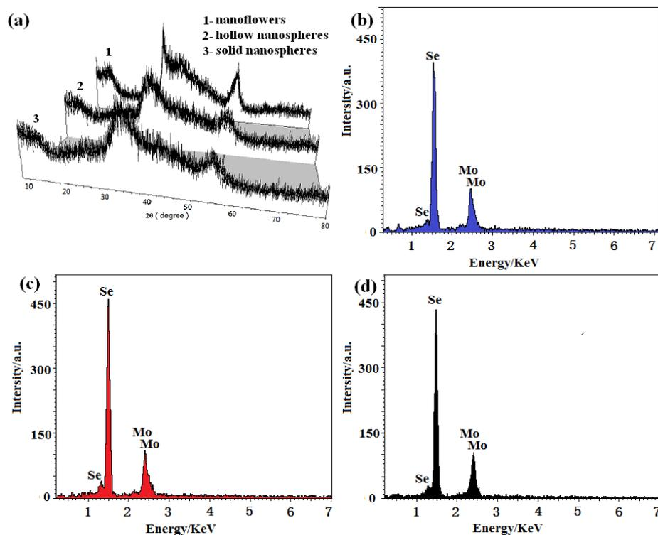
Fig. 1: (a) XRD pattern and (b-d) EDS of the prepared  $\text{MoSe}_2$  nanoflowers (Sample 1), hollow nanospheres (Sample 2) and solid nanospheres (Sample 3)
