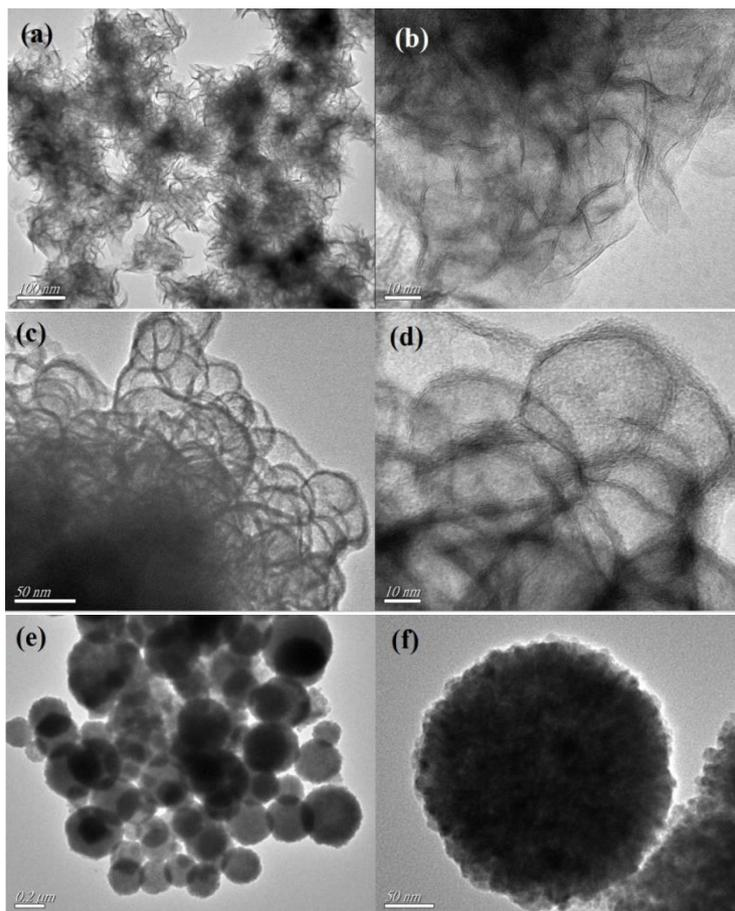
Fig. 2: TEM and HRTEM images of the prepared MoSe<sub>2</sub> (a and b) nanoflowers (Sample 1), (c and d) hollow nanospheres (Sample 2) and (e and f) solid nanospheres (Sample 3)
