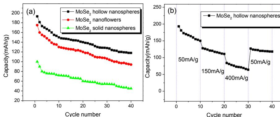
Fig. 3: (a) Cycle performances of the synthesized different MoSe<sub>2</sub> nanostructure at a constant current density of 50 mA g<sup>-1</sup>, (b) cycle performance of the MoSe<sub>2</sub> hollow nanospheres at different current density.
