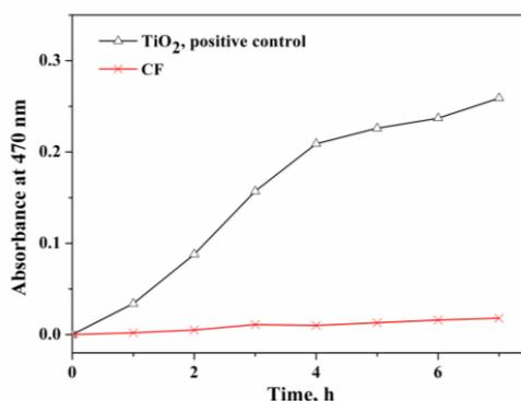
Fig. 5 Production of superoxide radical anion ( $O_2^{\cdot-}$ ) by CF dispersions. The  $O_2^{\cdot-}$  production was monitored during the incubation of XTT (0.4 mM) with CF (80  $\mu\text{g/mL}$ ) dispersions at pH 7.0 in dark. Incubation with  $\text{TiO}_2$  (40  $\mu\text{g/mL}$ ) under UV radiation was carried out as a positive control.
