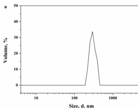
Fig. 2 Example of size distribution in the aqueous suspension of CF.
