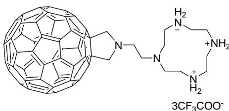
*Scheme 1 Molecular structures of the cyclen-functionalized fullerene derivatives, CF*
