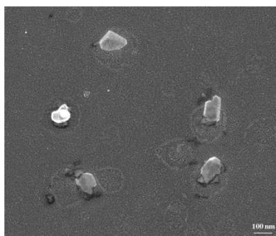
*Fig. 1 SEM micrographs of CF*
