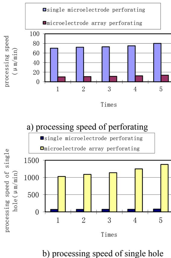
Fig. 5. Efficiency of micro-hole fabrication by single microelectrode and microelectrode array
