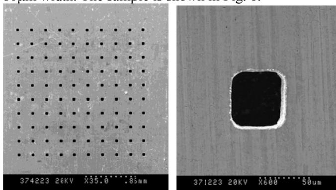
Fig. 6 SEM photographs of  $10 \times 10$  micro-hole array
