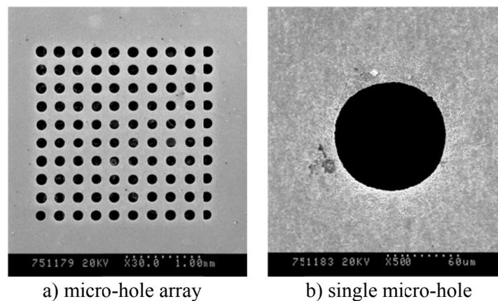
Fig.7. SEM photographs of example EMM machined.
