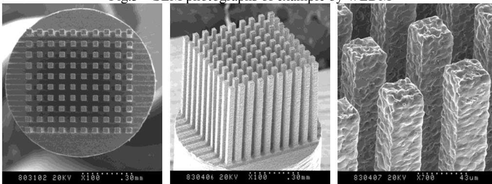
Fig. 4. SEM photographs of example by micro-WEDM.
