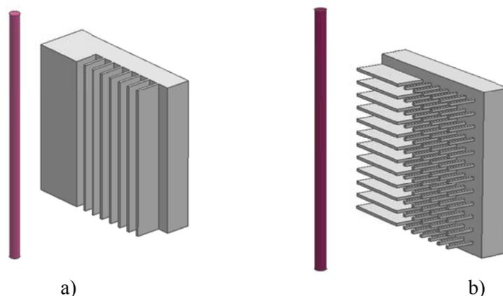
Fig.2 Sketch of microelectrode-array fabrication by WEDM.
