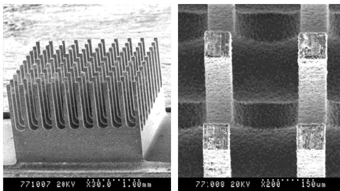
Fig.3 SEM photographs of example by WEDM
