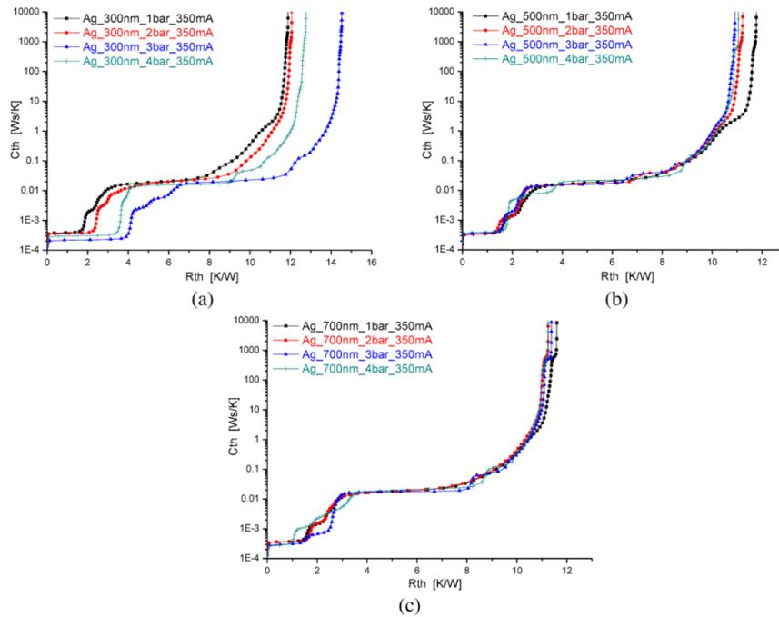
Fig. 3 Cumulative structure function curves of Ag thin film interfaced LED tested at various pressure for various Ag thin film thickness a) 300 nm, b) 500 nm and c) 700 nm
