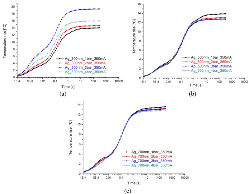
Fig. 1 Transient cooling curve of Ag thin film interfaced LED tested at various pressure for various Ag thin film thickness a) 300 nm, b) 500 nm and c) 700 nm
