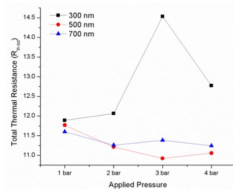
Fig. 4 Variation in total thermal resistance of LED at different thickness of Ag film for different applied pressure
