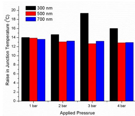
*Fig. 2 Variation in rise in junction temperature of LED at different thickness of Ag film for different applied pressure*
