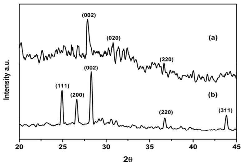
Fig.1 (a, b). The XRD pattern of CdS nano crystals on (a) unpolished and (b) chemically polished p-Si(100) substrates.
