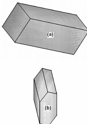
Fig. 2. (a, b). Calculated shape of the CdS nano crystals on (a) un polished and (b) chemically polished p-Si(100) substrate.
