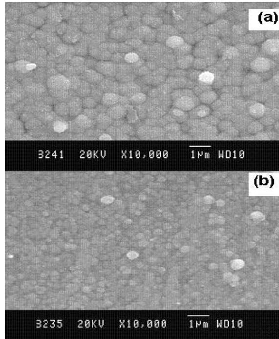
Fig.3 (a, b). The SEM images of CdS nano crystals on (a) unpolished and (b) chemically polished p-Si (100) substrates.
