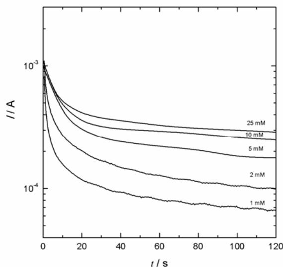
Fig. 6. Chronoamperometric curves of PANI enzyme electrode in glucose solution of 1, 2, 5, 10 and 25 mM.
