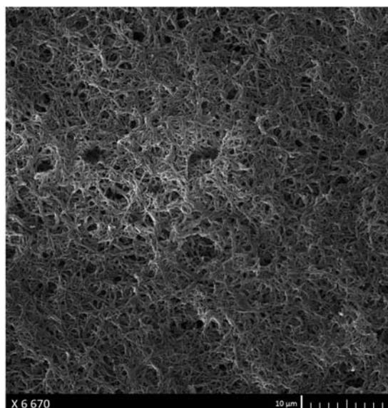
Fig. 4. SEM micrographs of the PANI electrochemically deposited onto graphite electrode.
