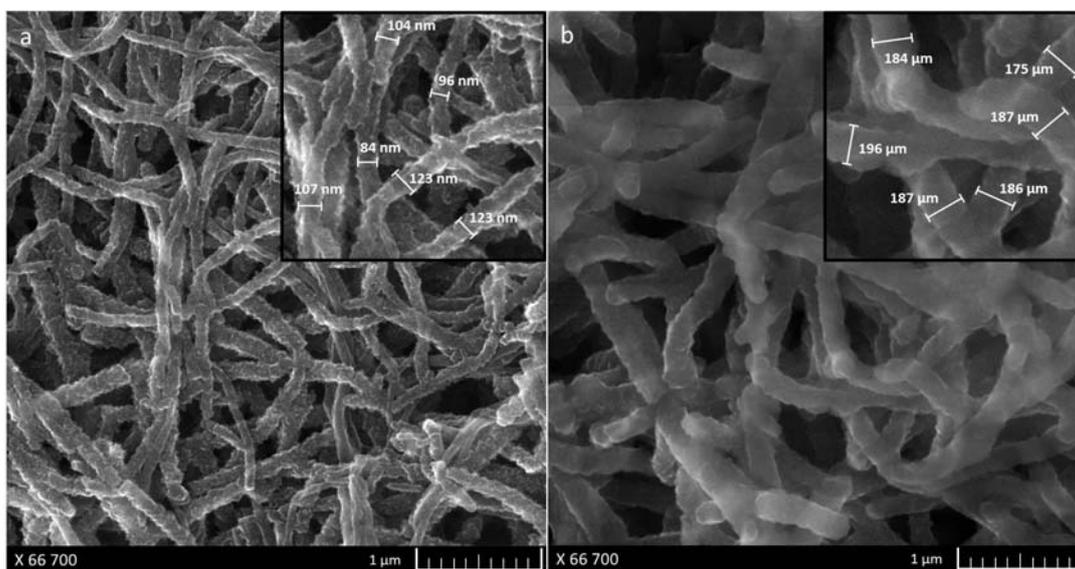
Fig. 5. a) SEM micrograph of the electrode surface a) before and b) after the immobilization. Inserts: enlarged part of the image for better visibility.
