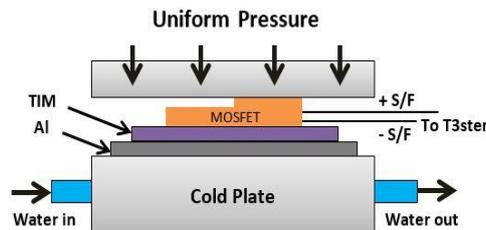
Fig. 2 Schematic diagram of Experimental setup
