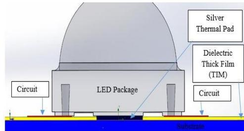
*Fig. 1: Schematic diagram of thick film substrate mounted with LED as a package via screen printing process.*
