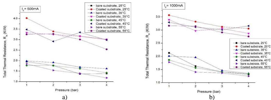
Fig. 3 Total thermal resistance of bare and coated substrates tested at different temperatures and pressure with driven current of a) 500mA b) 1000mA.
