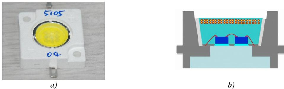
Fig. 1. (a) The white LED package without remote phosphor compound;
