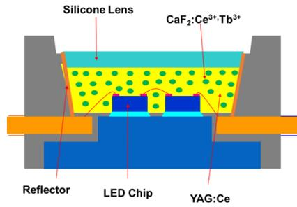
Fig. 1. The in-cup packaging WLEDs physical structure
