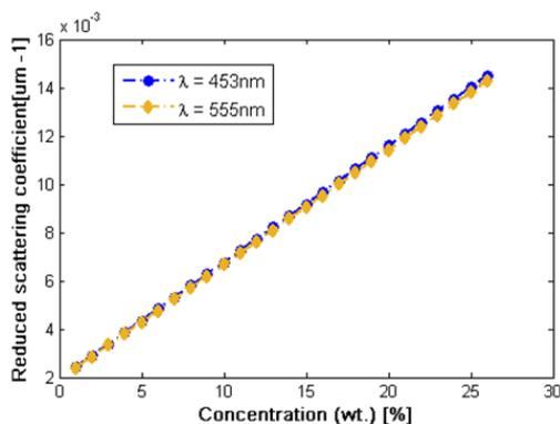
Fig. 3 The reduced scattering coefficient of the green-emitting  $\text{CaF}_2:\text{Ce}^{3+},\text{Tb}^{3+}$  phosphor at wavelengths of 453nm, 555nm.
