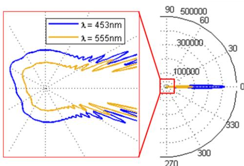
Fig. 4 The angular scattering amplitudes of the green-emitting  $\text{CaF}_2:\text{Ce}^{3+},\text{Tb}^{3+}$  phosphor at wavelengths of 453nm, 555nm.
